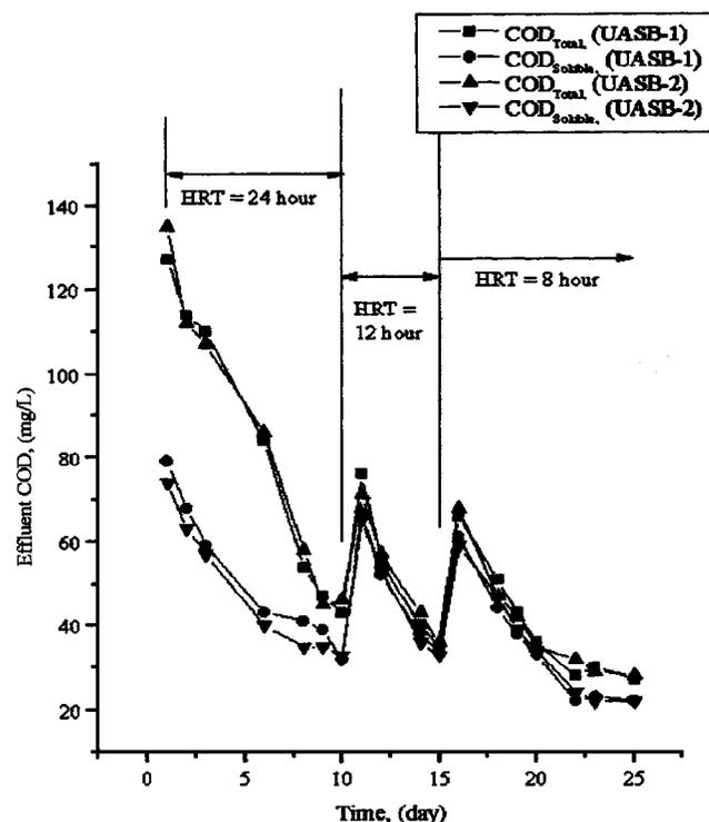
**Fig. 2.** Effluent chemical oxygen demand profile in upflow anaerobic sludge blanket reactors during startup period
