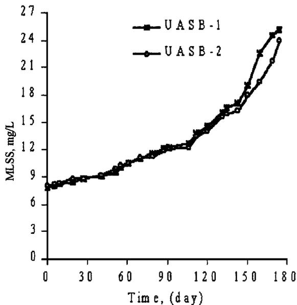
**Fig. 3.** Mixed liquor suspended solids profile of upflow anaerobic sludge blanket reactors treating various strength synthetic wastewaters
