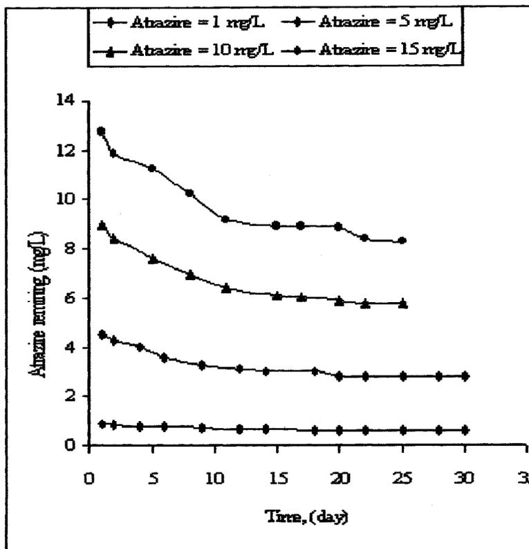
Fig. 4. Kinetics of atrazine reduction from wastewater with dextrose concentration of 150 mg/L
