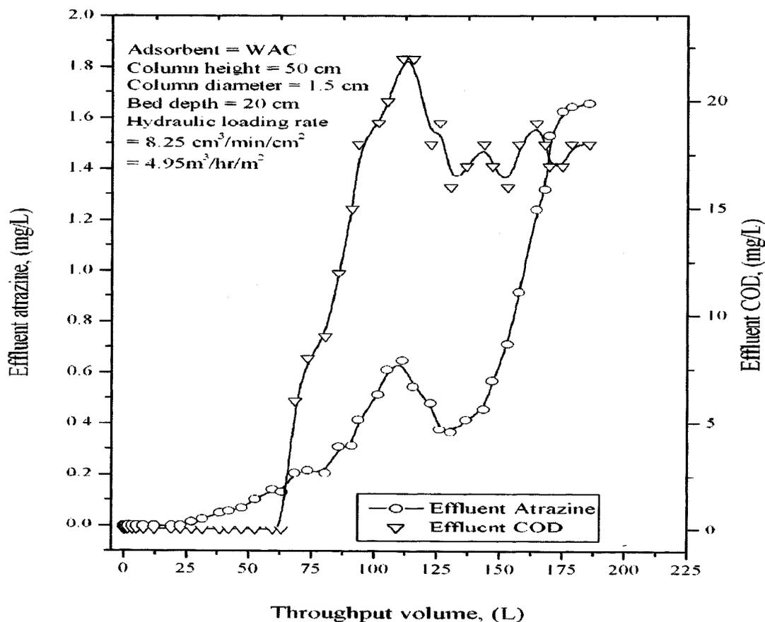
**Fig. 5.** Breakthrough curves for waste activated carbon removing atrazine and organic matter (chemical oxygen demand) in fixed bed adsorption column
