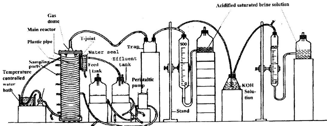
Fig. 1. Schematic diagram of laboratory scale setup of upflow anaerobic sludge blanket reactor
