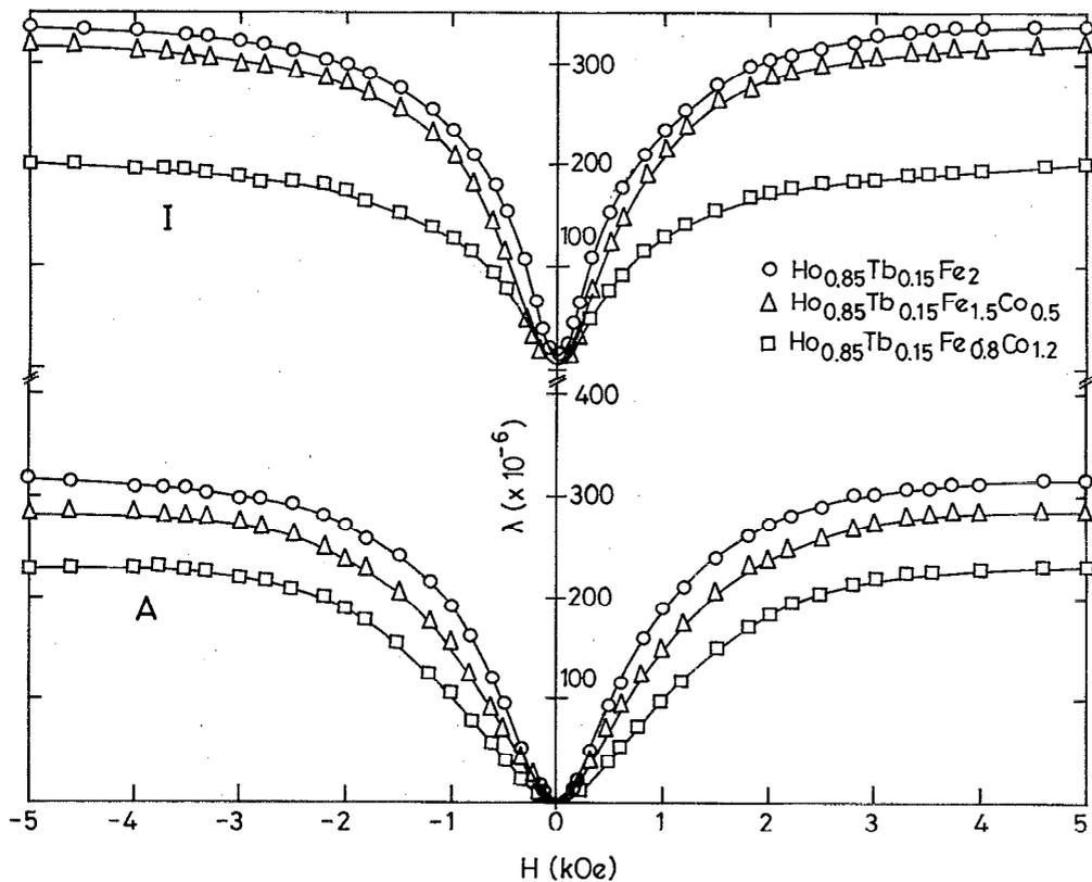
FIG. 1. Magnetostriction of *A* and *I* samples of  $\text{Ho}_{0.85}\text{Tb}_{0.15}\text{Fe}_{2-x}\text{Co}_x$  as a function of applied field at RT.
