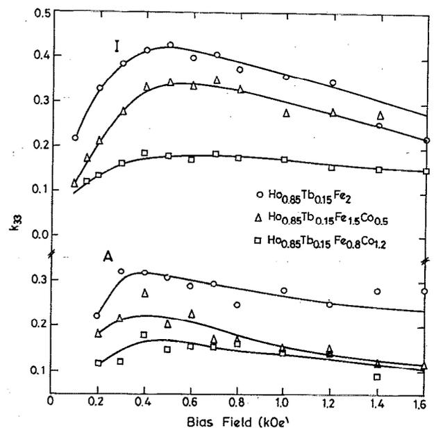
FIG. 3. Variation of  $k_{33}$  values for *A* and *I* samples of  $\text{Ho}_{0.85}\text{Tb}_{0.15}\text{Fe}_{2-x}\text{Co}_x$  with dc bias field.
