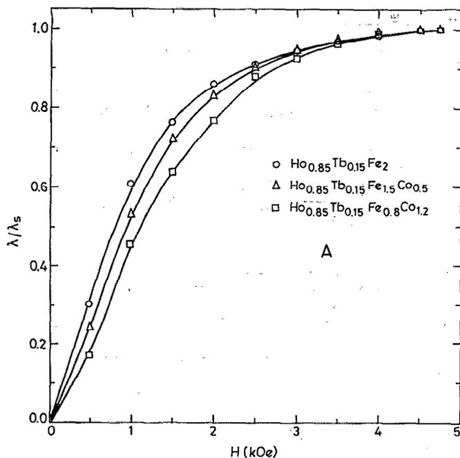
FIG. 4. Normalized magnetostriction as a function of applied bias field for *A* samples of  $\text{Ho}_{0.85}\text{Tb}_{0.15}\text{Fe}_{2-x}\text{Co}_x$ .
