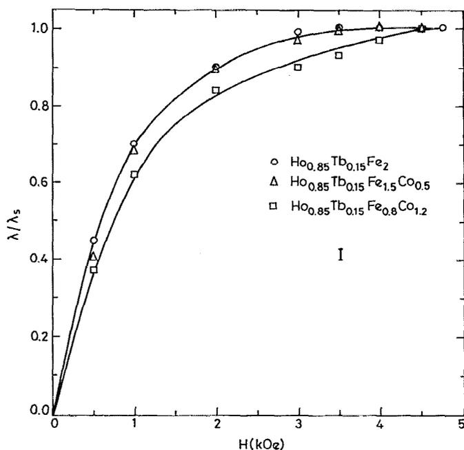
FIG. 5. Normalized magnetostriction as a function of applied bias field for *I* samples of  $\text{Ho}_{0.85}\text{Tb}_{0.15}\text{Fe}_{2-x}\text{Co}_x$ .
