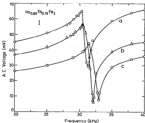
FIG. 2. Typical variation of resonant peaks with frequency for an *I* sample of  $\text{Ho}_{0.85}\text{Tb}_{0.15}\text{Fe}_2$  of 5.39-cm long. (a) 100 Oe, (b) 400 Oe, and (c) 1000 Oe.
