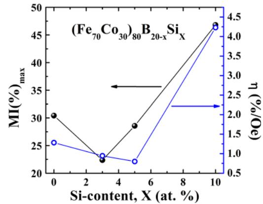
FIG. 7. Variation of  $\text{MI}(\%)_{\text{max}}$  and maximum field sensitivity ( $\eta$ ) with Si content for all  $(\text{Fe}_{70}\text{Co}_{30})_{80}\text{B}_{20-x}\text{Si}_x$  ribbons.
