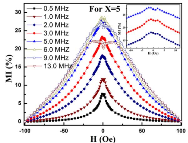
FIG. 4. Variation of MI(%) with magnetic field (H) for  $(\text{Fe}_{70}\text{Co}_{30})_{80}\text{B}_{15}\text{Si}_5$  ( $x=5$ ) ribbons. Inset: SP to DP transition at a low field range.
