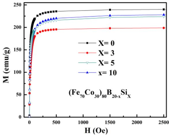
FIG. 1. M-H curves at 300 K for all  $(\text{Fe}_{70}\text{Co}_{30})_{80}\text{B}_{20-x}\text{Si}_x$  ribbons.
