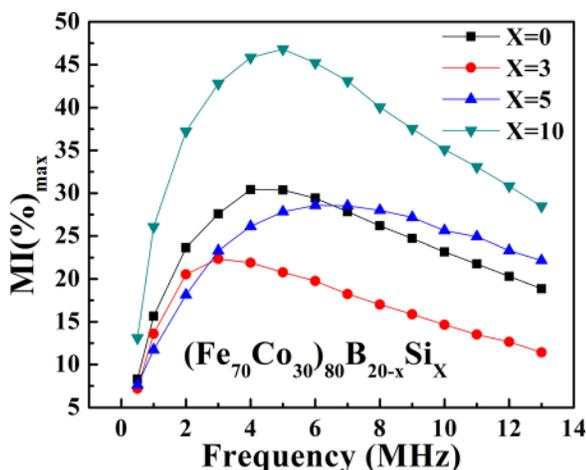
FIG. 6.  $\text{MI}(\%)_{\text{max}}$  variations with frequency for all  $(\text{Fe}_{70}\text{Co}_{30})_{80}\text{B}_{20-x}\text{Si}_x$  ribbons.
