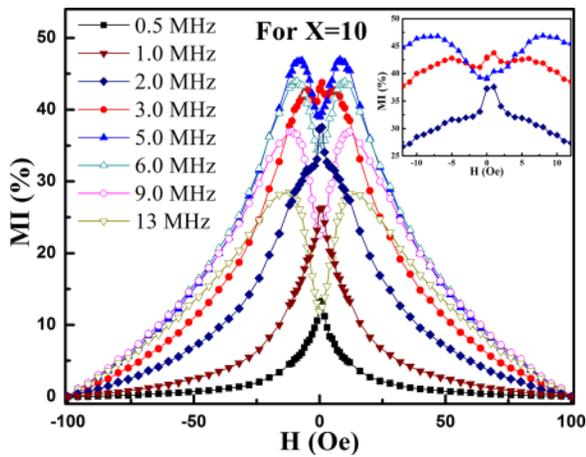
FIG. 5. Variation of MI(%) with magnetic field (H) for  $(\text{Fe}_{70}\text{Co}_{30})_{80}\text{B}_{10}\text{Si}_{10}$  ( $x = 10$ ) ribbons. Inset: SP to DP transition through TP at a low field range.
