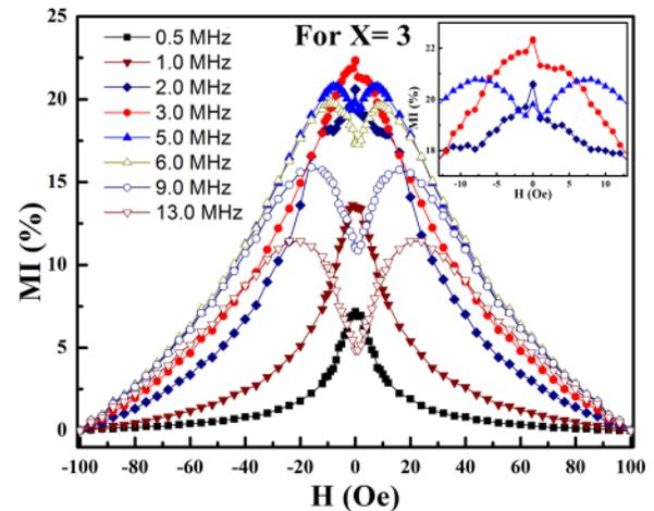
FIG. 3. Variation of MI(%) with magnetic field (H) for  $(\text{Fe}_{70}\text{Co}_{30})_{80}\text{B}_{17}\text{Si}_3$  ( $x=3$ ) ribbons. Inset: SP to DP transition through TP at a low field range.
