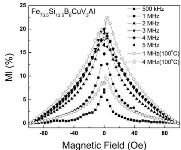
FIG. 3. Variation of  $MI$  with magnetic field for the as cast and annealed  $x = 0$  ribbon of 5 cm length at different frequencies.
