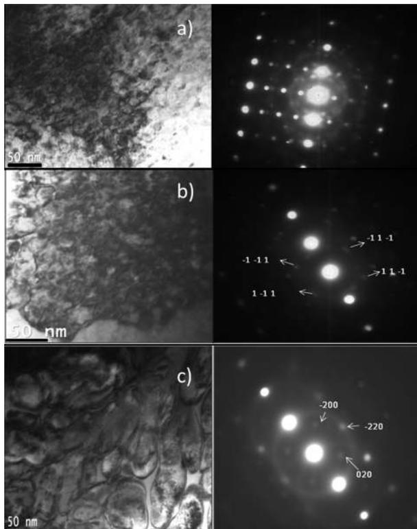
FIG. 2. TEM image (left) and diffraction pattern (right) of the as cast (a)  $x = 0$ , (b)  $x = 1.0$ , and (c)  $x = 1.5$  ribbons.
