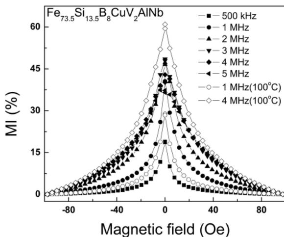
FIG. 4. Variation of  $MI$  with magnetic field for the as cast and annealed  $x = 1.0$  ribbon of 5 cm length at different frequencies.
