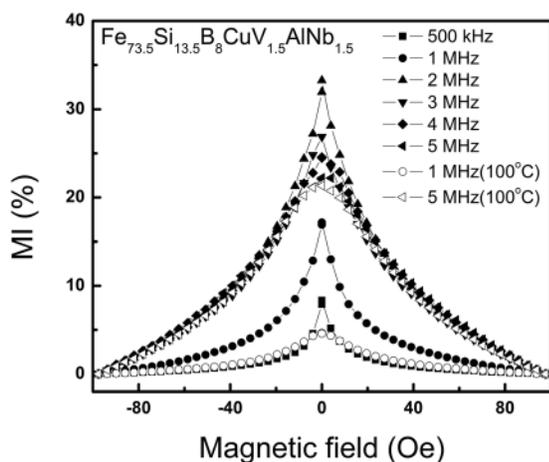
FIG. 5. Variation of  $MI$  with magnetic field for the as cast and annealed  $x = 1.5$  ribbon of 5 cm length at different frequencies.
