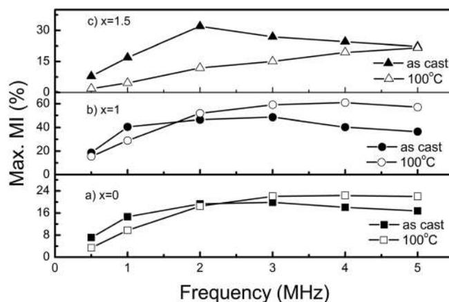
FIG. 6. Frequency variation of maximum  $MI$  for the as cast and annealed (a)  $x = 0$ , (b)  $x = 1$ , and (c)  $x = 1.5$  ribbons.
