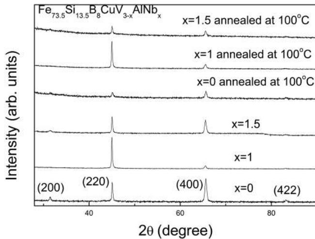
FIG. 1. XRD patterns of as cast and annealed  $\text{Fe}_{73.5}\text{Si}_{13.5}\text{B}_8\text{CuV}_{3-x}\text{AlNb}_x$  ( $x = 0, 1.0, 1.5$ ) ribbons.
