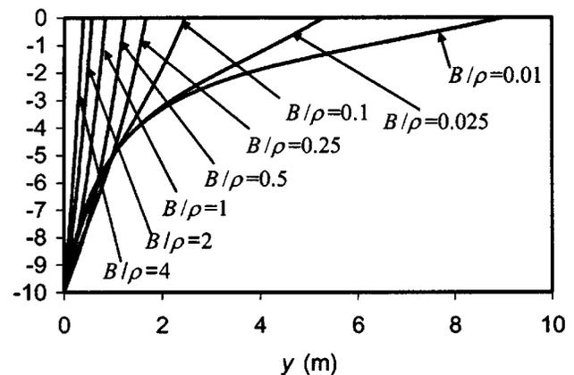
FIG. 1. Evolution of a compression wave front for various values of  $B/\rho$  for a linear density profile ( $\rho = 1 + y$ );  $|u_1(0)| = 0.1$ .
