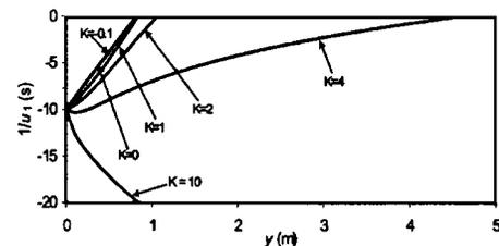
FIG. 3. Evolution of a compression wave front for various values of density gradient ( $K$ ) for a linear density profile ( $\rho=1+Ky$ ). The value of  $B/\rho$  is kept constant as 1;  $|u_1(0)|=0.1$ .
