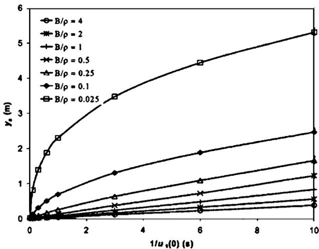
FIG. 2. The dependence of shock formation distance on the initial slope for various values of  $B/\rho$  for a linear density profile ( $\rho=1+y$ ).
