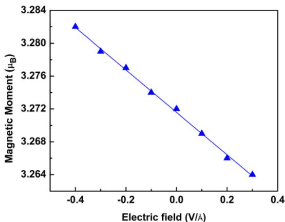
FIG. 2. The effect of an electric field on the magnetic moment of the Fe chain on Pt(001).
