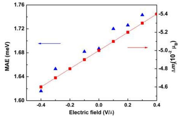
FIG. 3. Magnetic anisotropy energy (MAE, triangles) and orbital-moment anisotropy ( $\Delta m_l$ , squares) as a function of the electric field.
