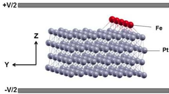
FIG. 1. Schematic of Fe chains on Pt(001) surface used in the present calculations.
