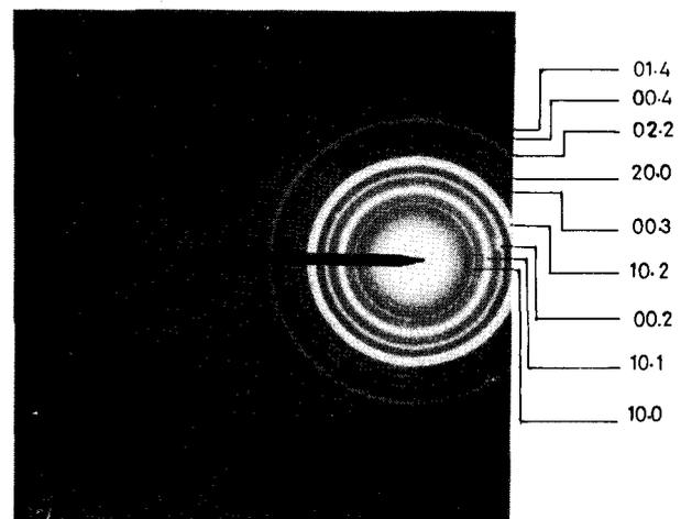
FIG. 1. Transmission electron diffraction pattern of a 500-Å-thick  $\text{MnSb}_{0.8}\text{Sn}_{0.2}$  film, taken at 80 kV. This shows that the film is composed of one phase of the NiAs structure.
