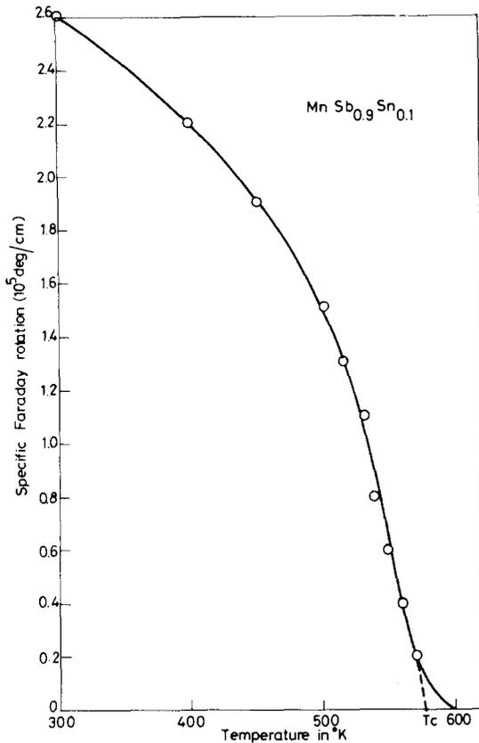
FIG. 4. Temperature dependence of specific Faraday rotation for a 450-Å-thick  $\text{MnSb}_{0.9}\text{Sn}_{0.1}$  film. The Curie temperature  $T_c$  is 575 K.
