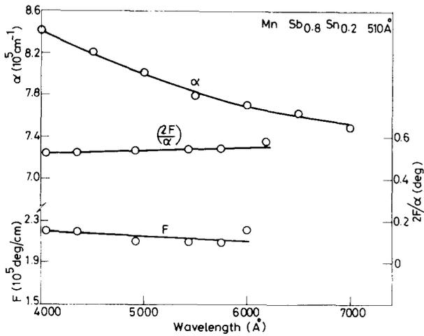
FIG. 2. Dispersion of specific Faraday rotation  $F$ , optical absorption coefficient  $\alpha$  and figure of merit  $(2F/\alpha)$  for  $\text{MnSb}_{0.8}\text{Sn}_{0.2}$  film. The thickness of the film was  $510 \text{ \AA}$ .
