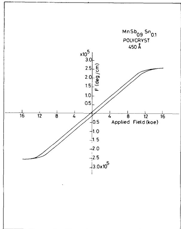
FIG. 3. Room-temperature polar Faraday rotation at  $6328 \text{ \AA}$  as a function of applied magnetic field.
