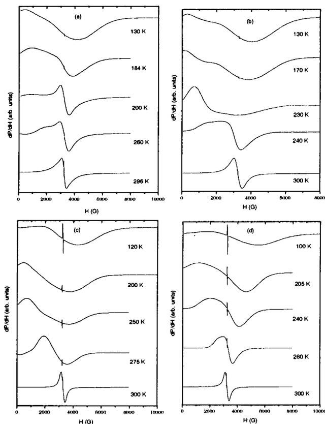
FIG. 1. ESR spectra of NSMO (a) 0.3, (b) 0.33, (c) 0.4, and (d) 0.5 for various temperatures.
