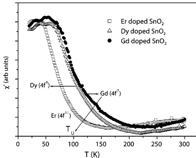
FIG. 2. Temperature variation of ac magnetic susceptibility of bulk RE-doped  $SnO_2$ .
