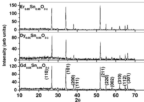
FIG. 1. X-ray diffractograms of polycrystalline  $Gd_{0.05}Sn_{0.95}O_{2-\delta}$ ,  $Dy_{0.05}Sn_{0.95}O_{2-\delta}$ , and  $Er_{0.05}Sn_{0.95}O_{2-\delta}$ .
