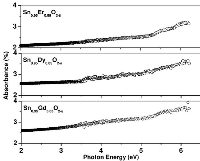
FIG. 3. Absorption spectra of rare earth doped thin films.
