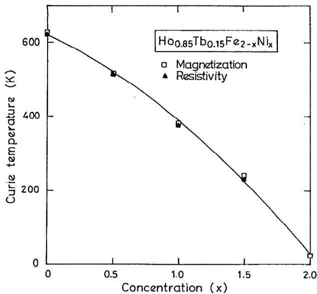
FIG. 4. Curie temperature as a function of  $x$  obtained from magnetization and resistivity measurements of  $\text{Ho}_{0.85}\text{Tb}_{0.15}\text{Fe}_{2-x}\text{Ni}_x$ . The value for  $x=2$  is taken as the weighted average of the  $T_C$  values of  $\text{HoNi}_2$  and  $\text{TbNi}_2$  from Ref. 4.
