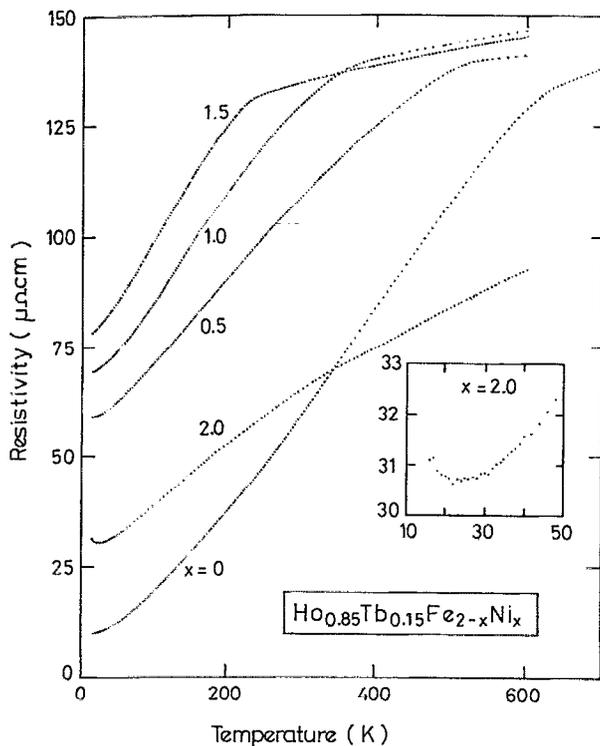
FIG. 5. Temperature variation of resistivity for various values of  $x$  of  $\text{Ho}_{0.85}\text{Tb}_{0.15}\text{Fe}_{2-x}\text{Ni}_x$ . The inset shows the anomaly observed for  $x=2$  in the vicinity of  $T_C$ .
