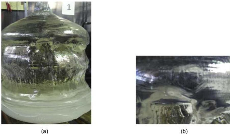
Fig. 1. Sapphire crystals obtained (a) by the Kyropolous method and (b) enlarged sapphire crystals.
