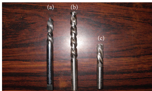
FIGURE 1: Tool used for machining. (a) Carbide D 5407060, (b) HSS twist drill (HSS-ORD, BS-328), and (c) HSS end mill (4 FLUTES “N”-type end mill RH-helical flute).
