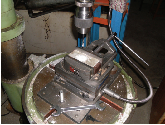
FIGURE 2: Kistler quartz three-component dynamometer (type 9257B).
