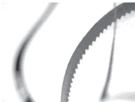
Fig. 8. SEM Micrographs showing saw tooth formation in chips
