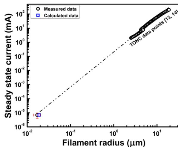
FIG. 3. Filament radius as a function of steady-state current in the *on* state, all the data points, except this work, were reproduced from the previous reports.<sup>13,14</sup> The filament radius (marked as square symbol) was calculated analytically based on the literature.<sup>18</sup> A very good agreement is obtained between the analytical value calculated with data and also consistent with the relationship of the steady state current is proportional to the square of filament radius.
