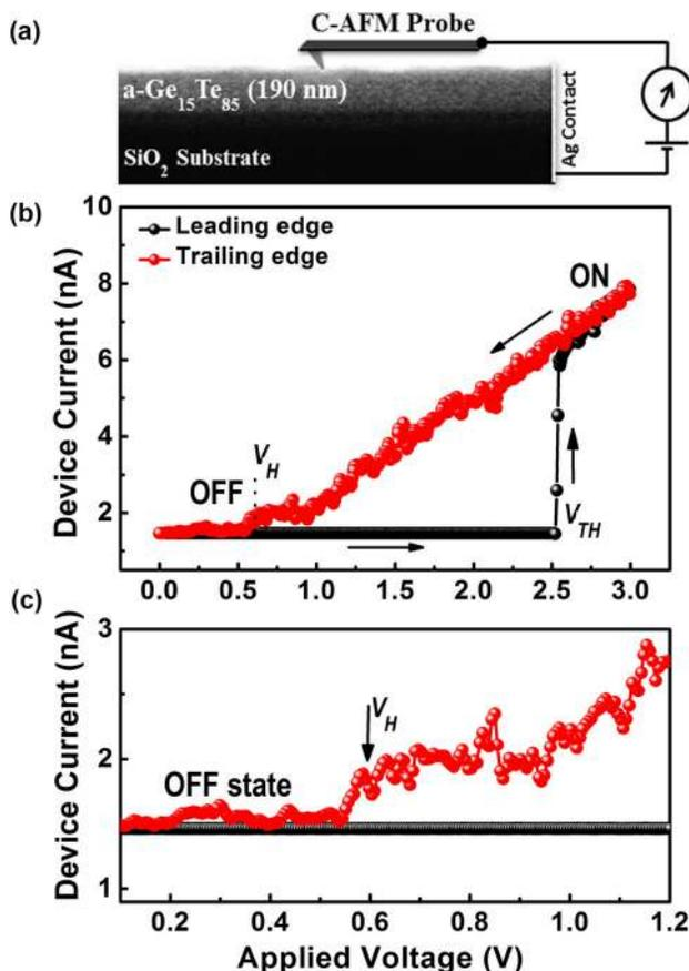
FIG. 1. (a) Schematic of C-AFM set-up used for performing the OTS behavior and *on-off* characteristics. (b) I-V characteristics and OTS behavior of GeTe<sub>6</sub> thin films for the applied electric voltage of 3 V. (c) Enlarged view of *on* to *off* transition via holding voltage  $V_H \sim 0.6 \pm 0.1$  V at which device current goes to zero.
