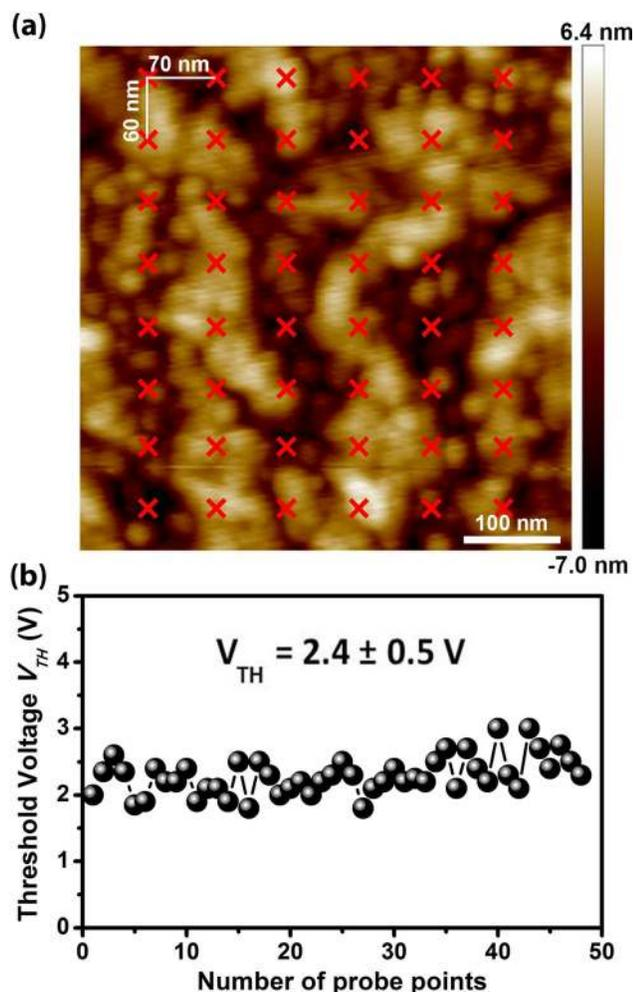
FIG. 2. (a) Surface morphology of a 500 nm region GeTe<sub>6</sub> thin films indicating 48 probe points at which threshold switching and *on-off* transitions were carried out by systematically varying 70 nm in X-direction and 60 nm in Y-direction. (b) Distribution of threshold voltage,  $V_{TH}$  of  $2.4 \pm 0.5$  V on 48 various probe points.
