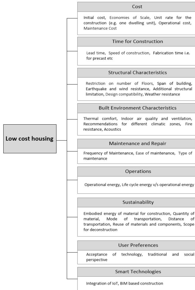
Figure 3. Criteria for evaluation of low-cost housing technologies
