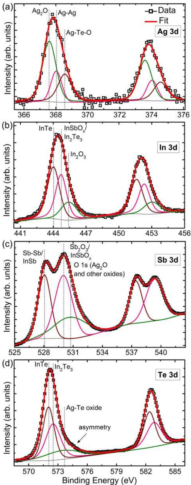
FIG. 1. XPS core level spectra of (a) Ag 3d, (b) In 3d, (c) Sb 3d, and (d) Te 3d, for as-deposited AIST.
