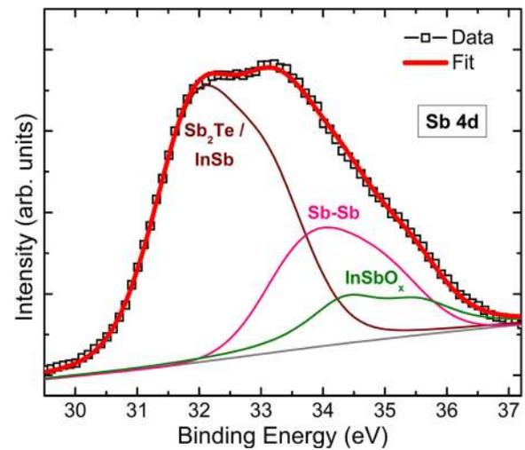
FIG. 2. XPS Sb 4d core level spectra for as-deposited AIST.
