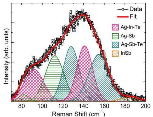
FIG. 3. Raman spectra for as-deposited AIST thin film.
