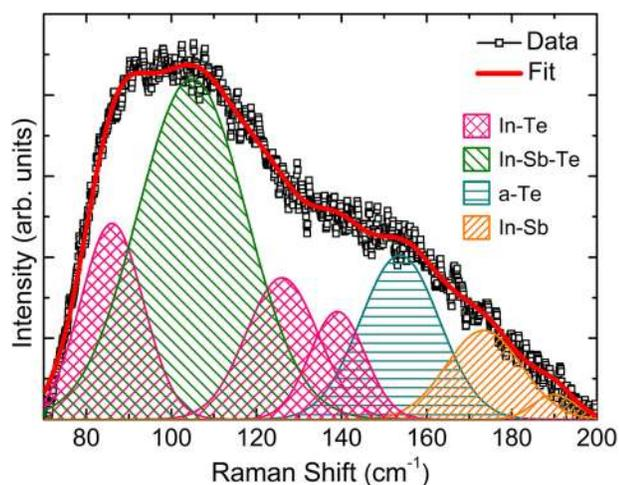
FIG. 6. Raman spectra for as-deposited IST thin film.
