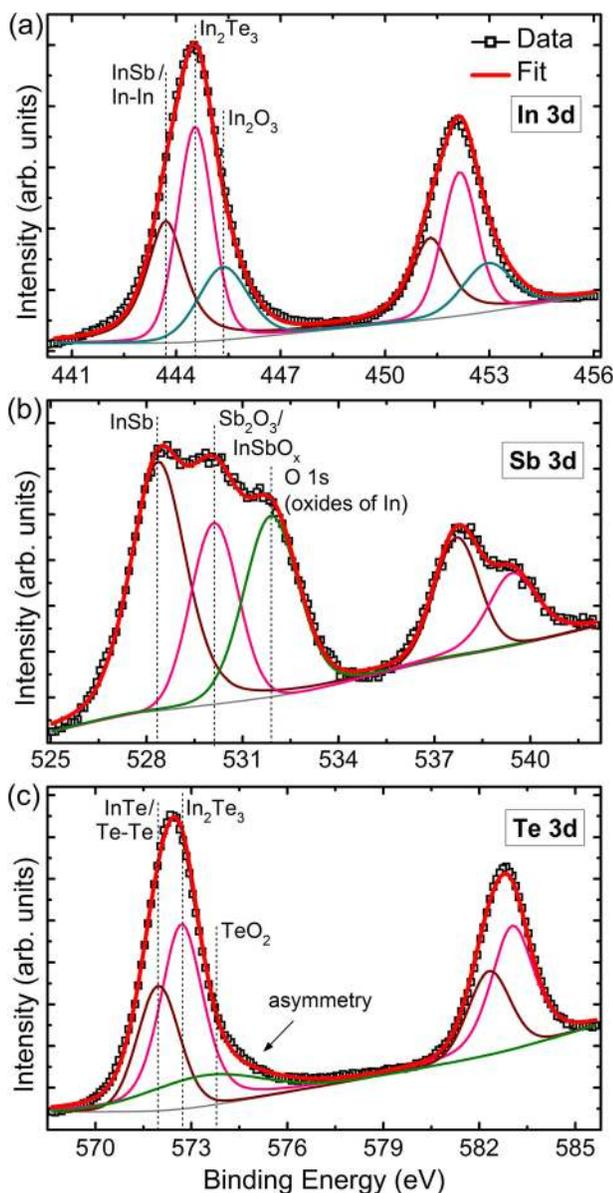
FIG. 4. XPS core level spectra of (a) In 3d, (b) Sb 3d, and (c) Te 3d, for as-deposited IST.
