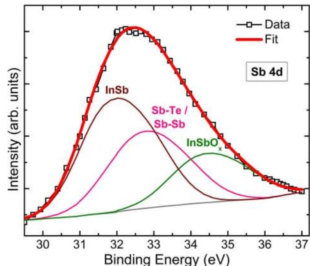
FIG. 5. XPS Sb 4d core level spectra for as-deposited IST.
