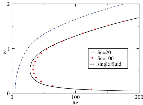
FIG. 3. Neutral stability boundaries of the surface mode for different Schmidt numbers when  $r = 0.4$ ,  $q = 0.2$ ,  $m = 1.5$ , and  $\theta = 10^\circ$ . The case of a single fluid<sup>21</sup> is also shown for comparison.
