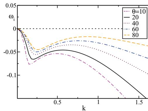
FIG. 10. Growth rate of the most unstable mode at a viscosity ratio  $m = 1.5$ , when  $Re = 15$ ,  $Sc = 1$ ,  $r = 0.4$ ,  $q = 0.2$ .
