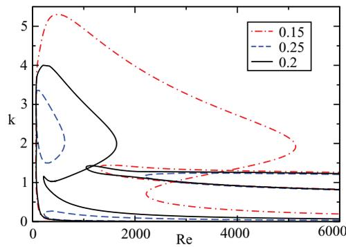
FIG. 16. Effect of changing the mixed-layer thickness  $q$  (in the legend) on the neutral boundaries of the overlap and TS modes. The other parameters are  $r = 0.5$ ,  $m = 1.5$ ,  $\theta = 10^\circ$ ,  $Sc = 20$ .
