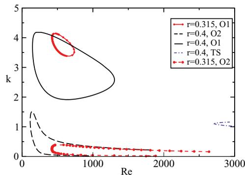
FIG. 6. Neutral boundaries of the O1, O2, and TS modes for different locations of the mixed layer when  $\theta = 10^\circ$ ,  $Sc = 20$ , and  $m = 1.5$ . Two distinct overlap modes are seen for smaller values of  $r$ . The Tollmien-Schlichting mode is seen at high Reynolds numbers and  $k \sim O(1)$  for  $r = 0.4$ . The surface mode is not shown in this figure.
