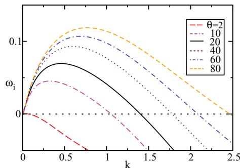
FIG. 11. Growth rate of the most unstable mode at a viscosity ratio  $m = 0.67$ , when  $Re = 15$ ,  $Sc = 1$ ,  $r = 0.4$ ,  $q = 0.2$ .
