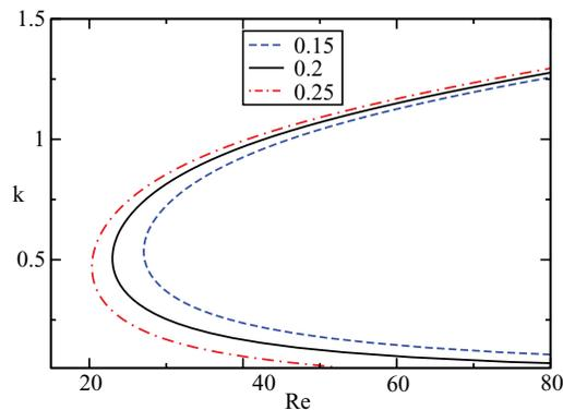
FIG. 17. Effect of changing the mixed-layer thickness  $q$  (in the legend) on the surface mode. Neutral boundaries are shown. The other parameters are  $r = 0.5$ ,  $m = 1.5$ ,  $\theta = 10^\circ$ ,  $Sc = 20$ .
