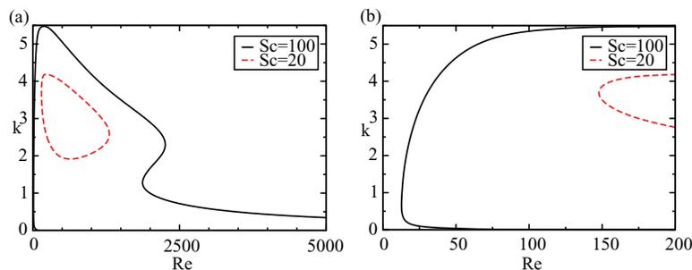
FIG. 4. (a) Neutral stability boundaries of the overlap mode O1 for different Schmidt numbers when  $r = 0.4$ ,  $q = 0.2$ ,  $m = 1.5$ . (b) The same, zoomed to low  $Re$ , to provide a comparison with the surface mode of Fig. 3.
