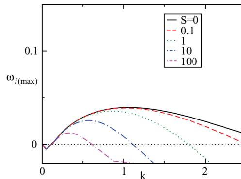
FIG. 13. Effect of surface tension, for different values of inverse capillary number  $S$ , for  $Re = 75$ ,  $m = 1.5$ . Here  $Sc = 10$ ,  $r = 0.4$ ,  $q = 0.2$ , and  $\theta = 10^\circ$ .
