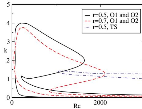
FIG. 7. Neutral boundaries of the overlap modes O1, O2, and TS modes for different locations of the mixed layer when  $\theta = 10^\circ$ ,  $Sc = 20$ , and  $m = 1.5$ . The two overlap modes merge together. The Tollmien-Schlichting mode is seen at high Reynolds numbers and  $k \sim O(1)$  for  $r = 0.5$ . The surface mode is not shown in this figure.
