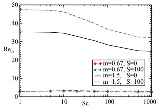
FIG. 15. Effects of surface tension on critical Reynolds number for two different viscosity ratios when  $r = 0.4$ ,  $q = 0.2$ , and  $\theta = 10^\circ$ .
