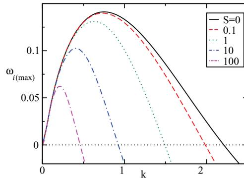
FIG. 14. Effect of surface tension, for different values of inverse capillary number  $S$ , for  $Re = 10$ ,  $m = 0.67$ . Here  $Sc = 10$ ,  $r = 0.4$ ,  $q = 0.2$ , and  $\theta = 10^\circ$ .
