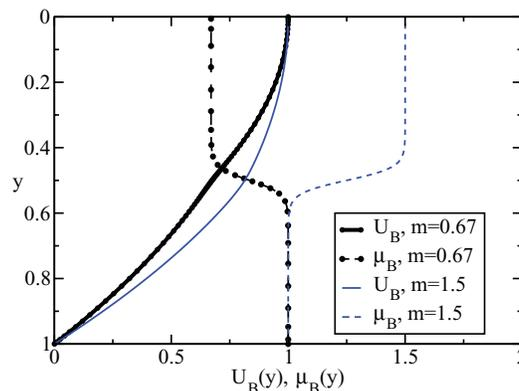
FIG. 2. Typical basic velocity and viscosity profiles. The interface is denoted by  $y = 0$  and the  $y$  coordinate increases to 1 at the wall.  $r$  and  $q$  are chosen to be 0.4 and 0.2, respectively, to place the mixed layer in the middle of the film.
