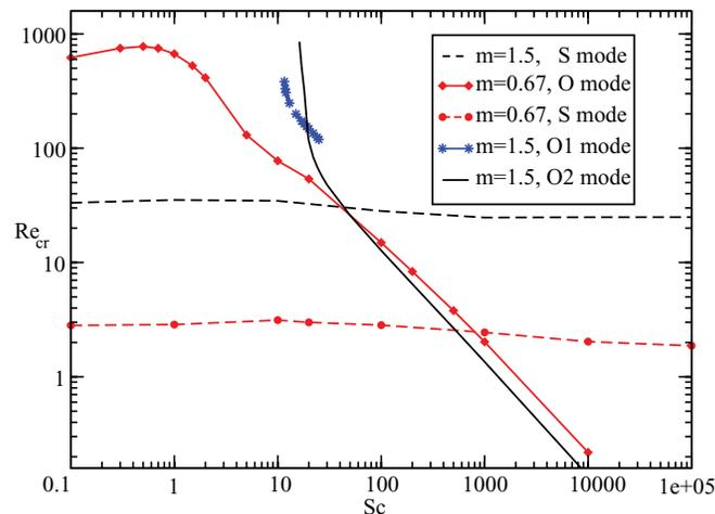
FIG. 8. Critical Reynolds number as a function of Schmidt number for  $r = 0.4$ ,  $q = 0.2$ , and  $\theta = 10^\circ$ .
