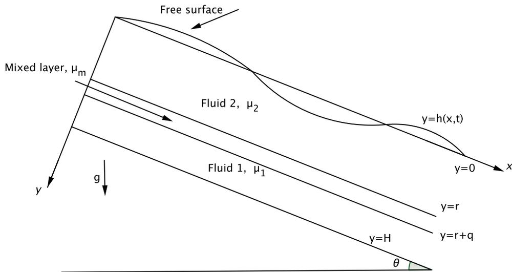
FIG. 1. Schematic of miscible two-layer flow down an inclined plane.
