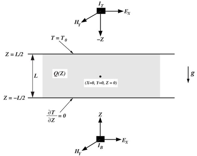
FIG. 1. Computational domain of oil layer confined between two horizontal plates exposed to microwave radiations of  $I_T$  and  $I_B$  from top and bottom, respectively. The coordinate system and the thermal boundary conditions are shown in the figure.
