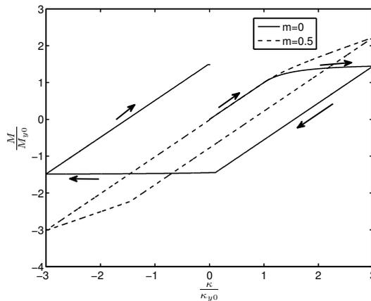
Fig. 2. Constitutive law for rectangular beam cross section
