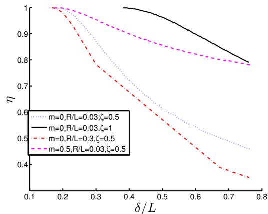
Fig. 4. Springback response for various process parameters
