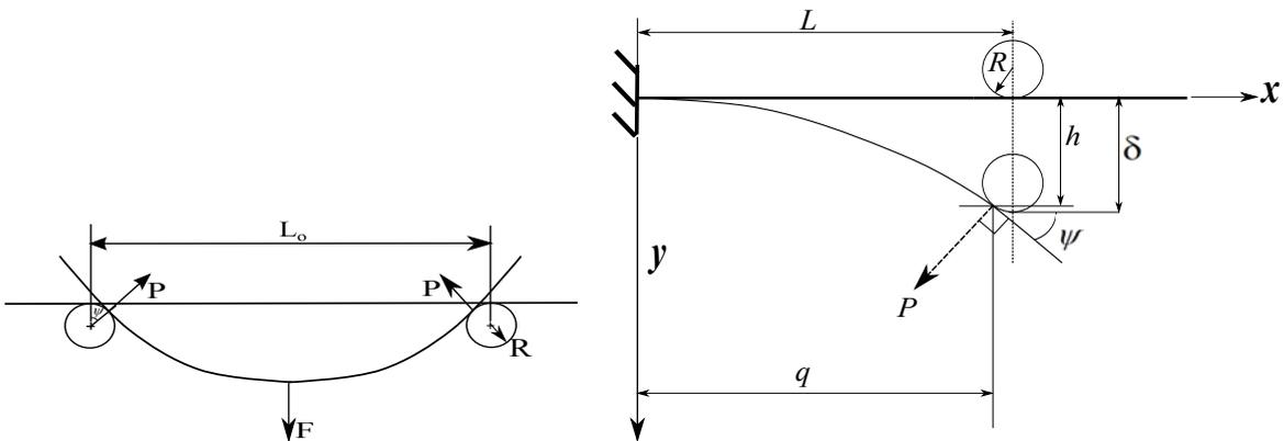
Fig. 1. Left: A long thin beam supported on finite dimensional cylindrical roller supports. Right:A long cantilever under friction-less roller punch induced large deflection
