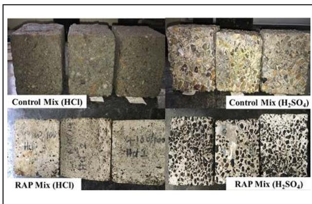
Figure 8. Specimens of control mix and RAP mix after exposure to attack by chloride and sulfate.
