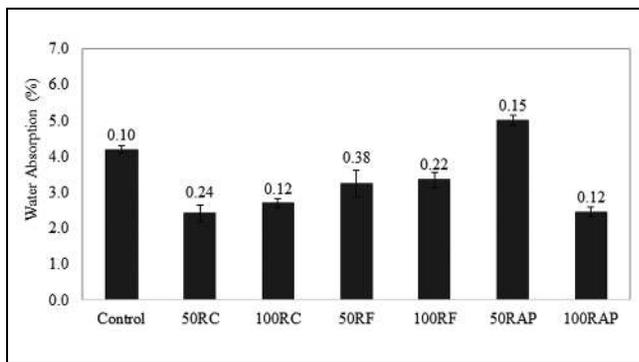
**Figure 6.** Water absorption of the RCCP mixes.
