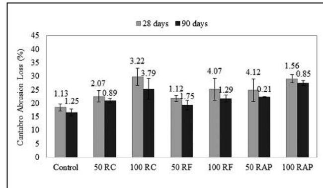
Figure 4. Cantabro abrasion loss of the RCCP mixes.
