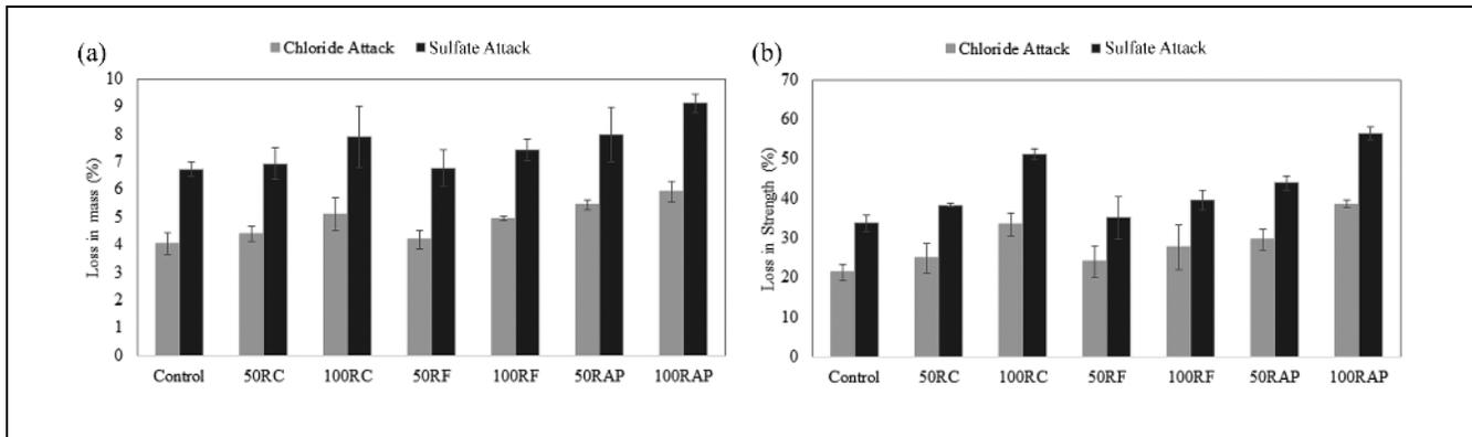
Figure 7. RAP mixes after exposure to aggressive environments: (a) loss in mass; (b) loss in strength.
