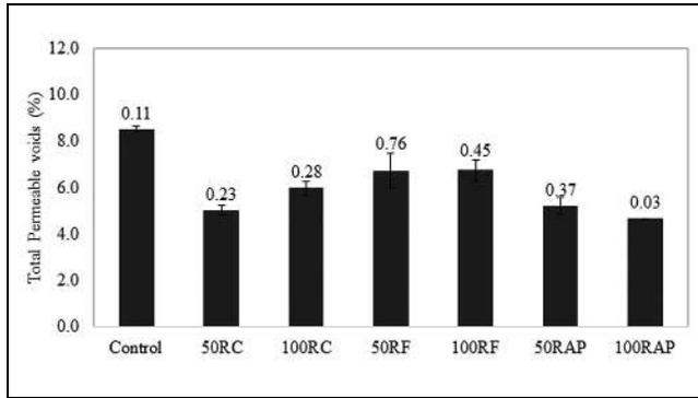
**Figure 5.** Total permeable voids of the RCCP mixes.
