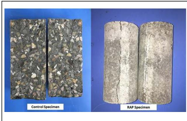
Figure 3. Split specimens after failure.
