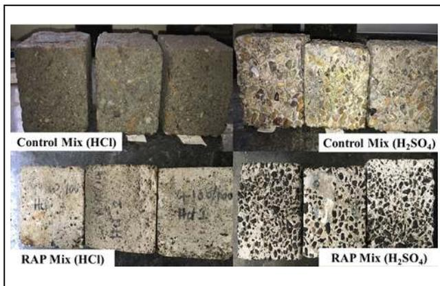
Figure 8. Specimens of control mix and RAP mix after exposure to attack by chloride and sulfate.
