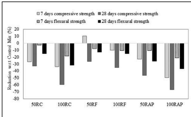
**Figure 2.** Reduction in strength of considered RAP mixes compared with control mix.
