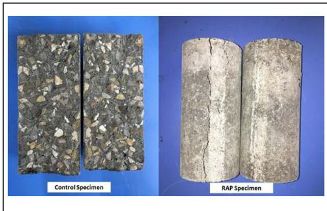
Figure 3. Split specimens after failure.
