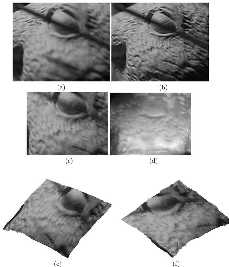
Fig. 6. (a,b) Observations of a clay model of a bunny occluded by a pin. (c) Inpainted focused image. (d) Estimated shape profile. (e, f) Novel views of the bunny.
