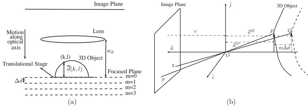
Fig. 3. (a) Working principle of SFF. (b) Schematic showing mechanism of structure-dependent pixel motion in SFF.
