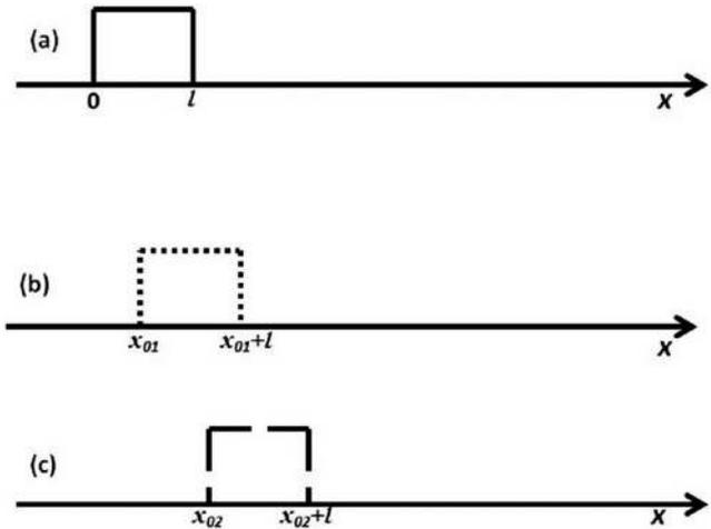
FIG. 1. The static strain pulse in the spatial domain at three different instants of time.
