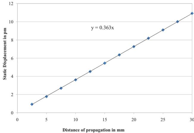
FIG. 3. (Color online) Variation in the static displacement with the distance of propagation for  $f=0.796$  MHz,  $\beta=30$ ,  $A=10$  nm,  $E=70$  GPa, and density of the material ( $\rho=2700$  kg/m<sup>3</sup>).
