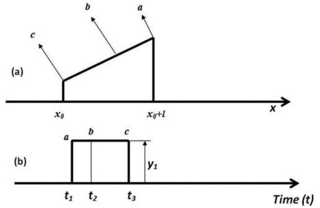
FIG. 2. (a) The static displacement pulse in the spatial domain. (b) The displacement pulse in the time domain as received at the receiver.
