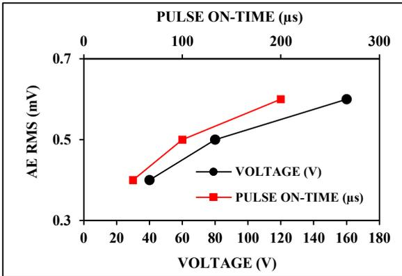
Fig. 6. (a) Comparison of AE RMS with voltage and pulse on-time
