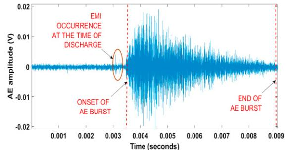
Fig 4. AE burst signal
