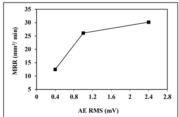
Fig. 7. (c) AE RMS vs. MRR
