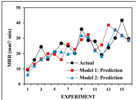
Fig. 8. (b) Predictability of MRR: Actual vs. Model 1 vs. Model 2
