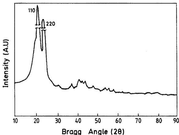
Fig. 4. Wide angle X-ray diffraction pattern of XLPE specimen.
