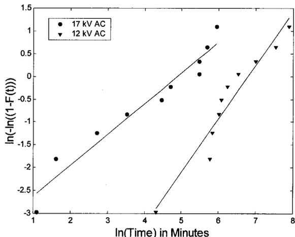
Fig. 2. Weibull plot of times to failure of XLPE specimen due to electrical tree under AC voltages.
