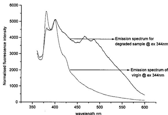
Fig. 6. Normalised emission spectrum of the degraded polymer.
