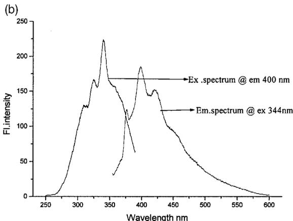
Fig. 7. Excitation emission spectrum of specimen after extraction with ether: (a) virgin sample; (b) tree followed with breakdown zone.
