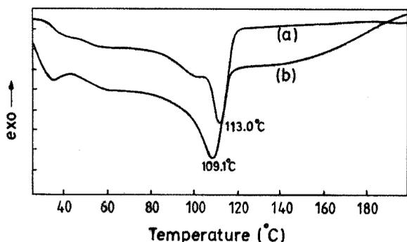
Fig. 5. DSC thermogram: (a) virgin sample; (b) tree followed with breakdown zone sample.
