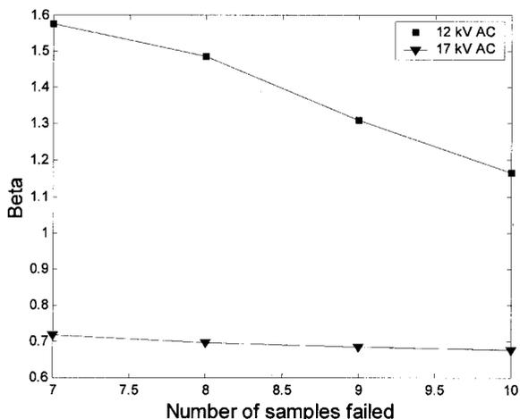
Fig. 3. Variation in the shape parameter ( $\beta$ ) with number of samples failed in an experimental run.
