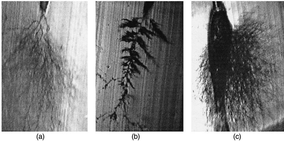
Fig. 1. Electrical trees under AC voltage: (a) bush type tree; (b) tree-like tree; (c) tree followed with breakdown.
