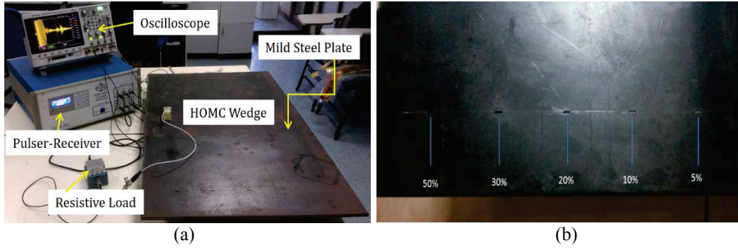
FIGURE 2. Photograph of (a) experimental setup; (b) Plate showing the machined notches as a percentage of thickness.
