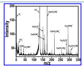
**Figure 3.** Mass spectrum of ACN- $h_3$ :H<sub>2</sub>O mixture obtained on 1 keV Cs<sup>+</sup> ion collision.
