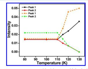
**Figure 9.** Maximum intensity of fitted (Lorentzian fit) free (peak 1) and H-bonded (peak 2)  $C \equiv N$  stretching frequency of ACN- $h_3$ :H<sub>2</sub>O (solid line) and ACN- $d_3$ :H<sub>2</sub>O (dotted line) is plotted against temperature.
