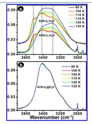
**Figure 2.** Temperature-dependent RAIRS spectra in the OH stretching region of (a) 1:1 codeposited ACN- $h_3$ :H<sub>2</sub>O and ACN- $d_3$ :H<sub>2</sub>O and (b) layer-on-layer ACN- $h_3$ @H<sub>2</sub>O on cold Ru(0001) surface at 40 K.
