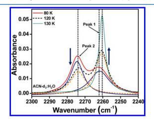
**Figure 7.** Lorentzian fit of the spectra of  $1:1 \text{ ACN-}d_3:\text{H}_2\text{O}$  at three different temperatures. Both fitted and cumulative spectra are shown in the figure. Two peaks in the cumulative spectra at each temperature are fitted with two components, peak 1 corresponds to the free ACN molecules and peak 2 corresponds to H-bonded ACN molecules. Fitted spectrum and cumulative spectrum were overlapping at 130 K. Hence, only fitted spectrum is shown in the figure at 130 K.
