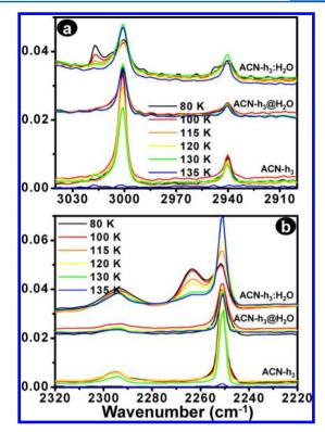
**Figure 4.** (a) Enlarged view of C–H asymmetric and symmetric stretching regions and (b) C $\equiv$ N stretching region of ACN- $h_3$  of pure acetonitrile, ACN- $h_3$ :H<sub>2</sub>O, and ACN- $h_3$ @H<sub>2</sub>O at different temperatures.
