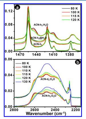
**Figure 5.** Temperature-dependent RAIRS spectra in (a) bending mode of C–H bond of ACN, ACN- $h_3$ :H<sub>2</sub>O, and ACN- $d_3$ :H<sub>2</sub>O mixtures and (b) O–D stretching mode of codeposited ACN- $h_3$ :D<sub>2</sub>O and ACN- $d_3$ :D<sub>2</sub>O mixtures.
