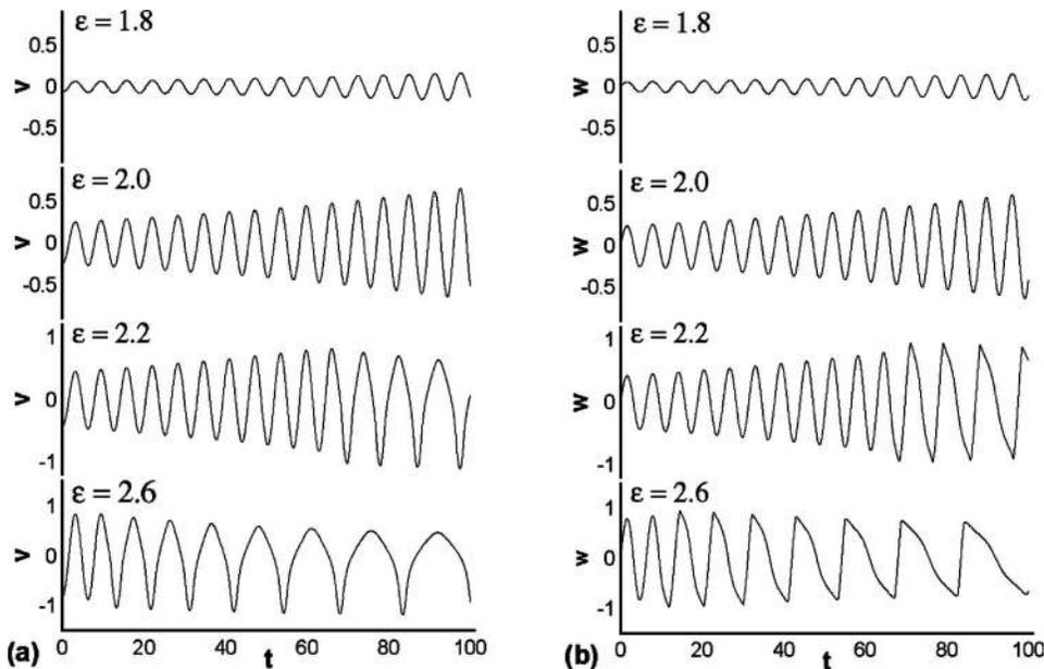
FIG. 9. Transverse velocity of a fluid particle for parallel counter-rotating Rankine vortices with different axial separations ( $x_0=0.0, y_0=0.0, z_0=2.0; t=100$ ) with a superimposed uniform velocity in the  $x$  direction ( $u_0=0.05$ ): (a)  $y$  component of velocity and (b)  $z$  component of velocity.
