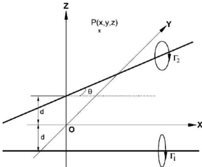
FIG. 1. Configuration of two skewed and inclined Rankine vortices with a viscous core.
