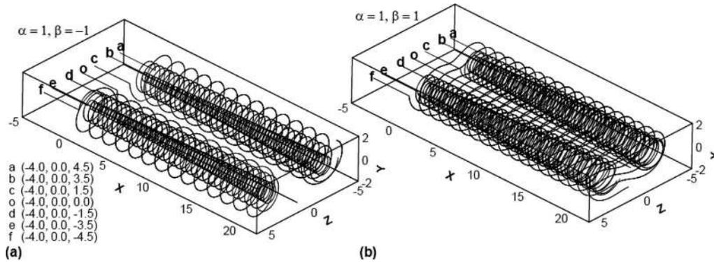
FIG. 12. Path of six different fluid particles entering a confined channel ( $H/a=4.0$ ) in the  $x$  direction ( $u_0=0.05$ ) in the field of parallel semi-infinite Rankine vortices with axial separation of  $\varepsilon=3.0$ : (a) counter-rotating and (b) corotating.
