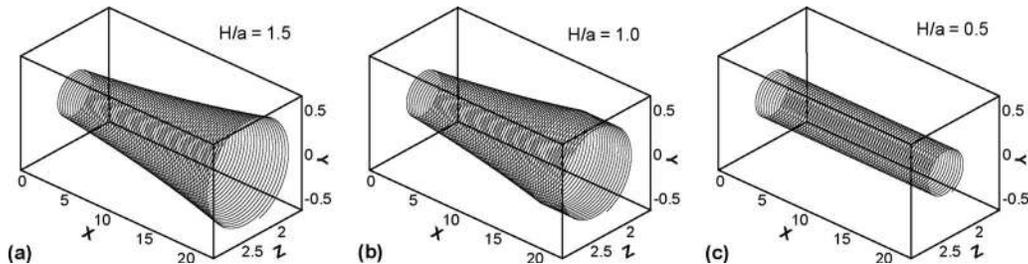
FIG. 10. Path of a fluid particle for parallel skewed counter-rotating Rankine vortices ( $x_0=0.0, y_0=0.0, z_0=2.0; t=500$ ) with a superimposed uniform velocity in the  $x$  direction ( $u_0=0.05$ ) for different confinements: (a)  $H/a=1.5$ , (b)  $H/a=1.0$ , and (c)  $H/a=0.5$ .
