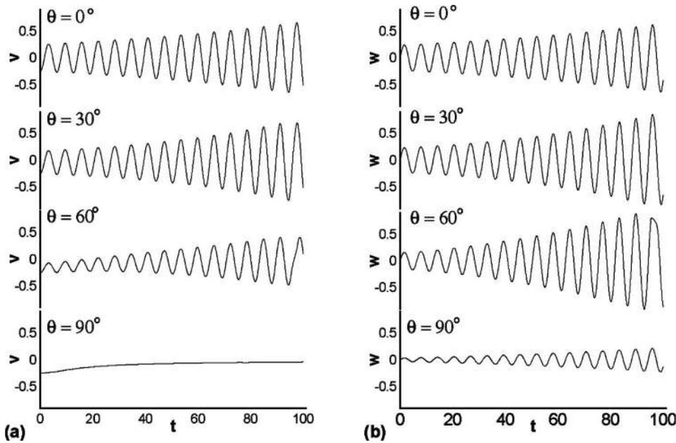
FIG. 7. Transverse velocity signal of a fluid particle for four different angular orientations of the skewed Rankine vortices ( $\alpha=1.0$ ,  $\beta=-1.0$ ,  $\varepsilon=2.0$ ,  $u_0=0.05$ ;  $x_0=0.0$ ,  $y_0=0.0$ ,  $z_0=2.0$ ;  $t=100$ ) with a superimposed uniform velocity in the  $x$  direction: (a)  $y$  component of velocity and (b)  $z$  component of velocity.
