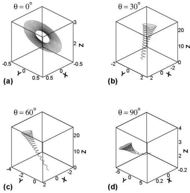
FIG. 4. Path of a fluid particle for four different angular orientations of the skewed Rankine vortex pair ( $\alpha=1.0$ ,  $\beta=-1.0$ ,  $\varepsilon=2.0$ ;  $x_0=0.0$ ,  $y_0=0.0$ ,  $z_0=2.0$ ;  $t=100$ ).
