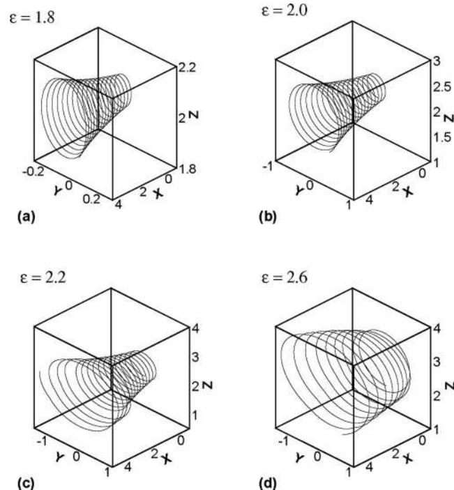
FIG. 8. Path of a fluid particle for parallel counter-rotating Rankine vortices with different axial distances ( $x_0=0.0$ ,  $y_0=0.0$ ,  $z_0=2.0$ ;  $t=100$ ) with a superimposed uniform velocity in the  $x$  direction ( $u_0=0.05$ ).
