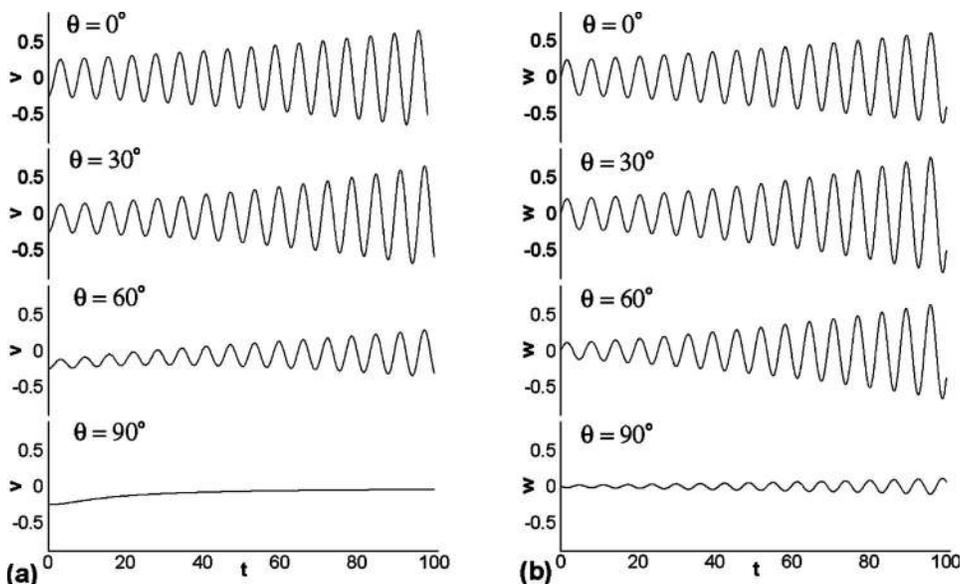
FIG. 5. Transverse velocity signal of a fluid particle for four different angular orientations of the skewed Rankine vortex pair ( $\alpha=1.0$ ,  $\beta=-1.0$ ,  $\varepsilon=2.0$ ;  $x_0=0.0$ ,  $y_0=0.0$ ,  $z_0=2.0$ ;  $t=100$ ): (a)  $y$  component of velocity and (b)  $z$  component of velocity.
