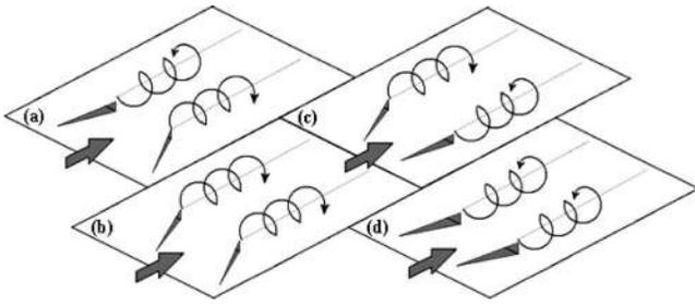
FIG. 2. Longitudinal fixed vortex filaments generated by winglet-type vortex generators mounted on a fin plate: (a)  $\alpha=1$ ,  $\beta=-1$ , (b)  $\alpha=1$ ,  $\beta=1$ , (c)  $\alpha=-1$ ,  $\beta=1$ , and (d)  $\alpha=-1$ ,  $\beta=-1$ .
