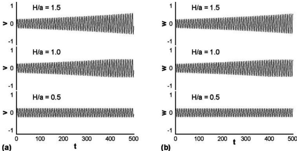
FIG. 11. Velocity of a fluid particle for parallel skewed counter-rotating Rankine vortices ( $x_0=0.0, y_0=0.0, z_0=2.0; t=500$ ) with translational velocity in the  $x$  direction ( $u_0=0.05$ ) with different confinements.
