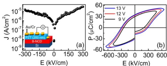
FIG. 2. Leakage current density ( $J$ ) versus electric field ( $E$ ) characteristics of the PLD grown PZT thin film on the conducting B-NCD substrate; the inset schematic illustrates the setup used to test the ferroelectric properties of the PZT/B-NCD capacitor. (b) Polarization ( $P$ ) versus applied electric field ( $E$ ) hysteresis loops of the sample with different applied voltages.
