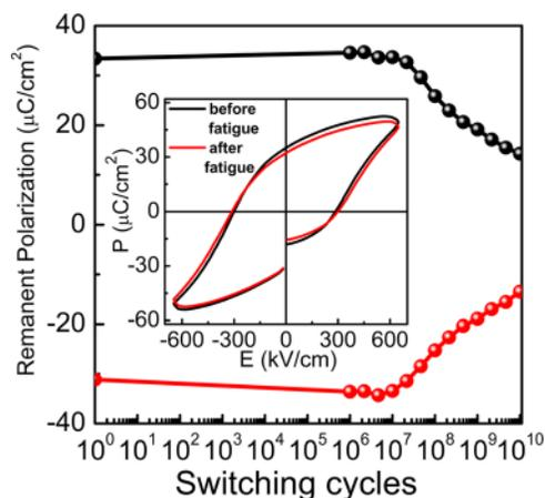
FIG. 4. Remanent polarization as functions of cumulative polarization switching cycles. The inset shows the hysteresis (P-E) loops before and fatigued states after being subjected to  $10^{10}$  switching cycles of the PLD grown PZT thin films on a conducting B-NCD substrate.
