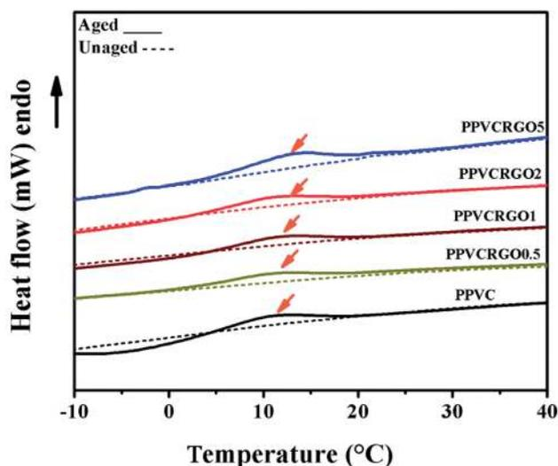
Fig. 8 Physical aging of PPVC/RGO nanocomposites at  $T_a = -10$  °C during 15 h.
