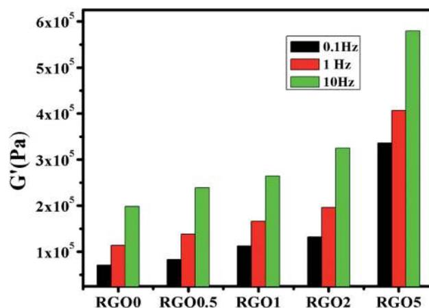
Fig. 4 Variations of storage modulus with filler loading.
