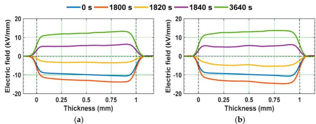
**Figure 11.** Electric field distribution under polarity reversal from positive to negative DC field stress in (a) virgin and (b) 8 kGy gamma irradiated specimens [29].
