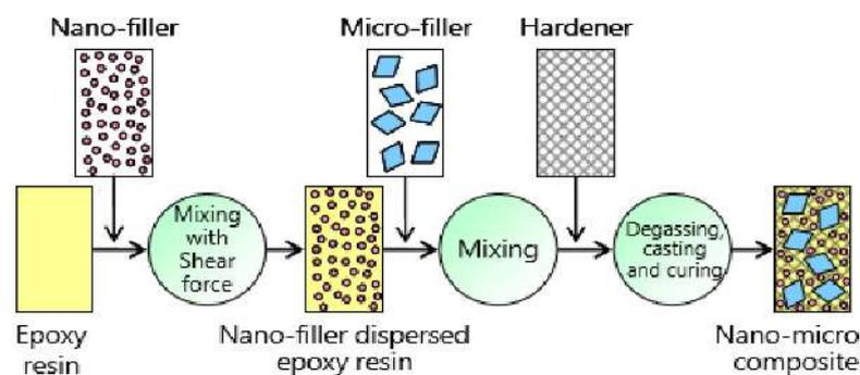
**Figure 1.** Scheme for the preparation of epoxy micro-nanocomposites [30].
