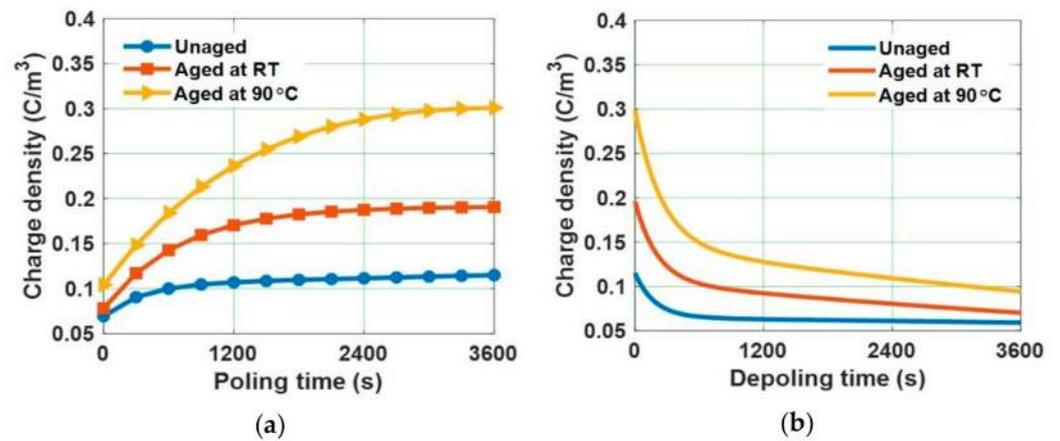
Figure 16. Mean value of absolute space charge density in water aged samples during (a) poling time and (b) depoling time [30].
