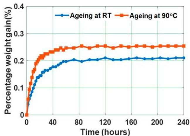
Figure 2. Percentage weight gain of epoxy samples subjected to water ageing at room temperature (RT) and 90 °C [30].
