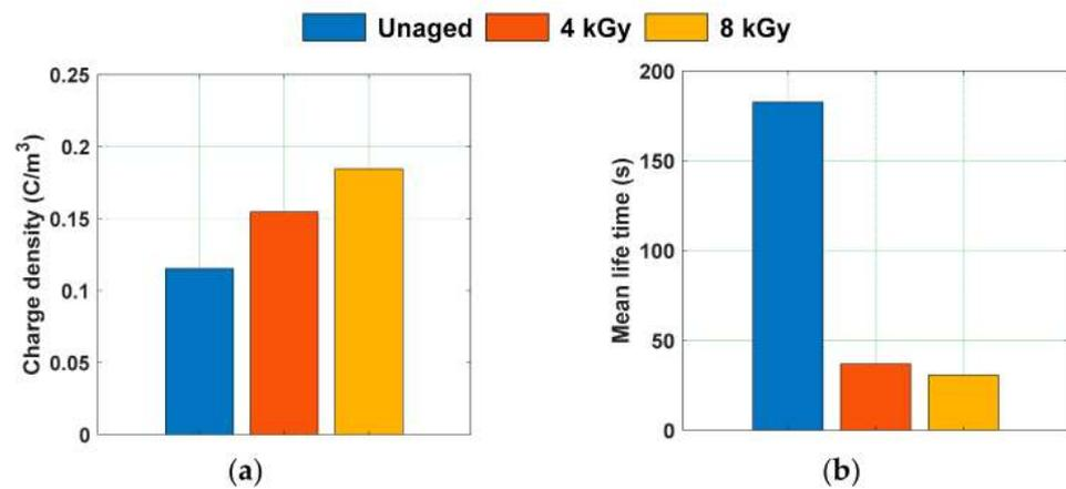
**Figure 9.** (a) Initial charge density just before depoling and (b) mean lifetime of space charge decay of gamma irradiated samples.
