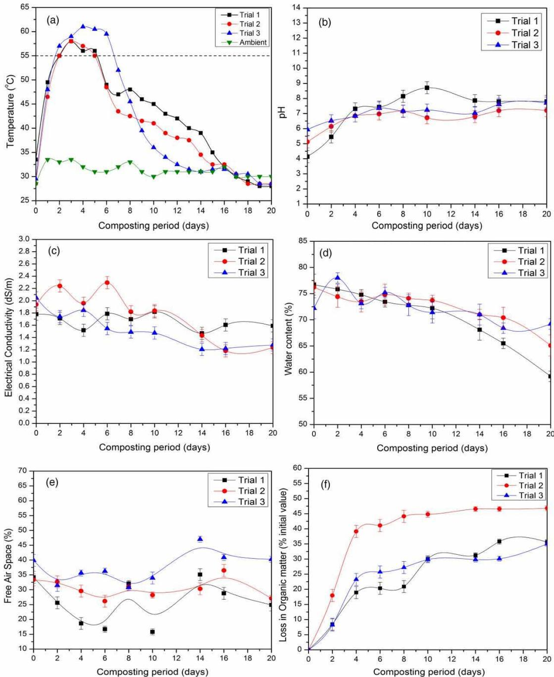
**Figure 2** | Change in composting parameters (a) temperature profile; (b) pH; (c) EC; (d) water content; (e) FAS (f) loss of organic matter; (g) loss in total nitrogen; (h) ammonia-nitrogen; (i) nitrate-nitrogen; (j) total phosphorous; (k) potassium; (l) C/N ratio. (continued).
