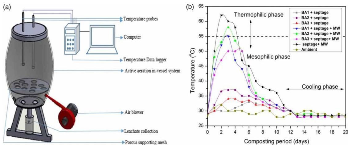
**Figure 1** | (a) Experimental set-up of in-vessel co-composting system; (b) Temperature profiles of trials with combination of various BAs, septage and MW. BA1: straw; BA2: coir pith; BA3: bagasse.
