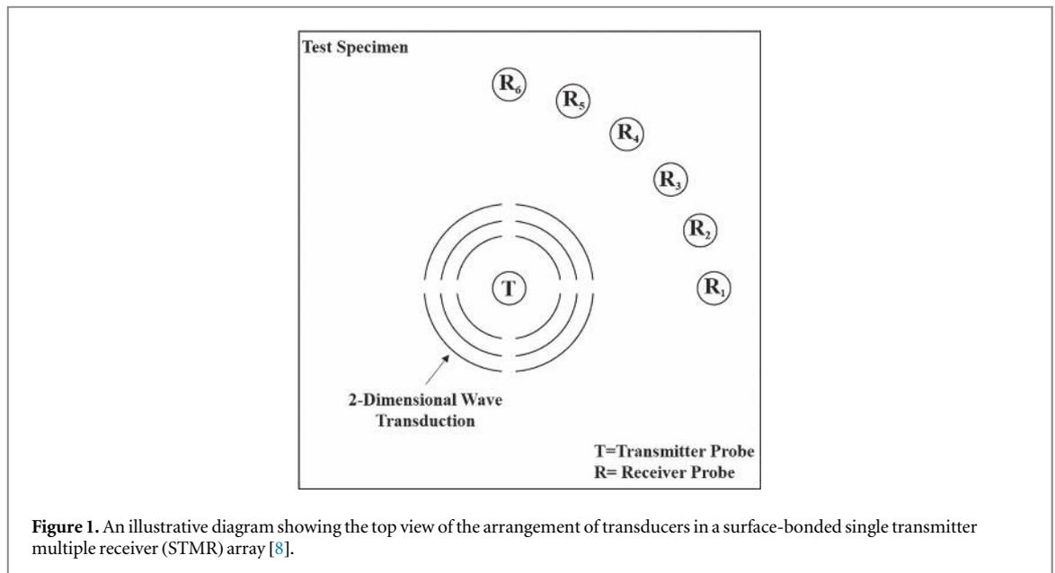
**Figure 1.** An illustrative diagram showing the top view of the arrangement of transducers in a surface-bonded single transmitter multiple receiver (STMR) array [8].
