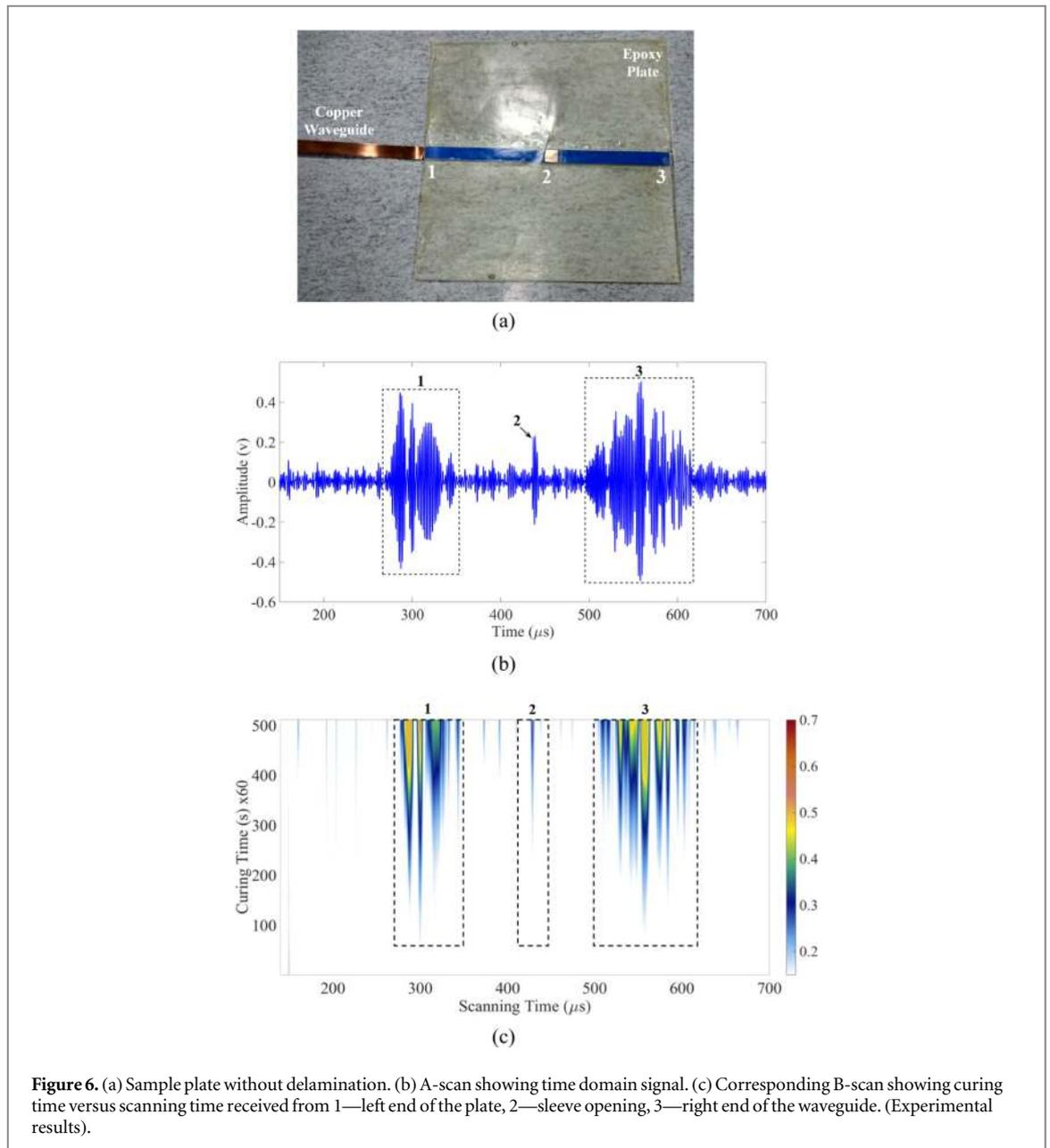
**Figure 6.** (a) Sample plate without delamination. (b) A-scan showing time domain signal. (c) Corresponding B-scan showing curing time versus scanning time received from 1—left end of the plate, 2—sleeve opening, 3—right end of the waveguide. (Experimental results).
