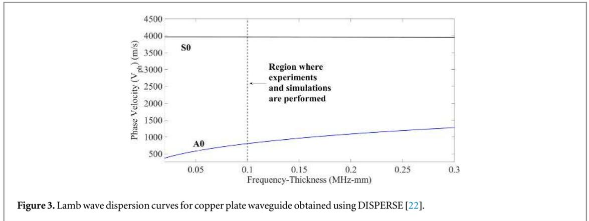
Figure 3. Lamb wave dispersion curves for copper plate waveguide obtained using DISPERSE [22].
