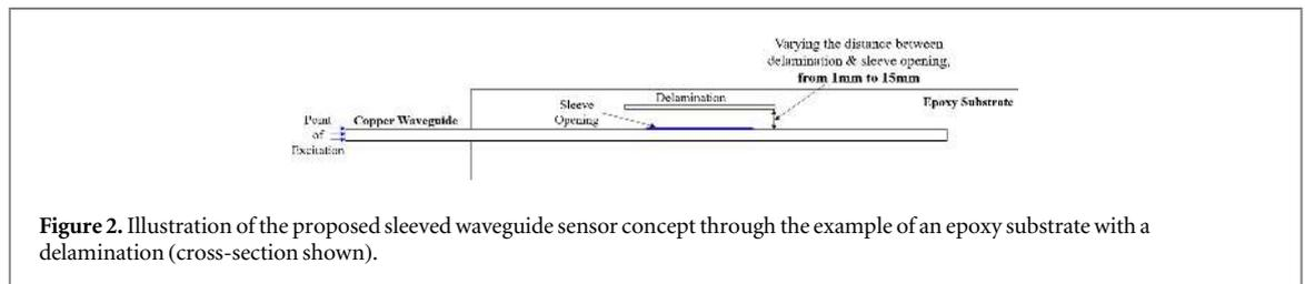
**Figure 2.** Illustration of the proposed sleeved waveguide sensor concept through the example of an epoxy substrate with a delamination (cross-section shown).
