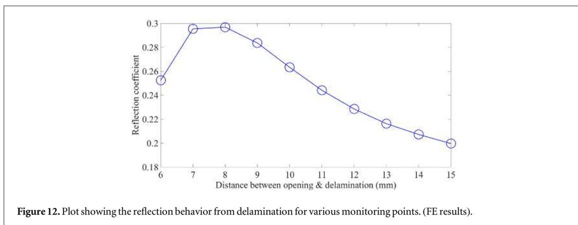
Figure 12. Plot showing the reflection behavior from delamination for various monitoring points. (FE results).
