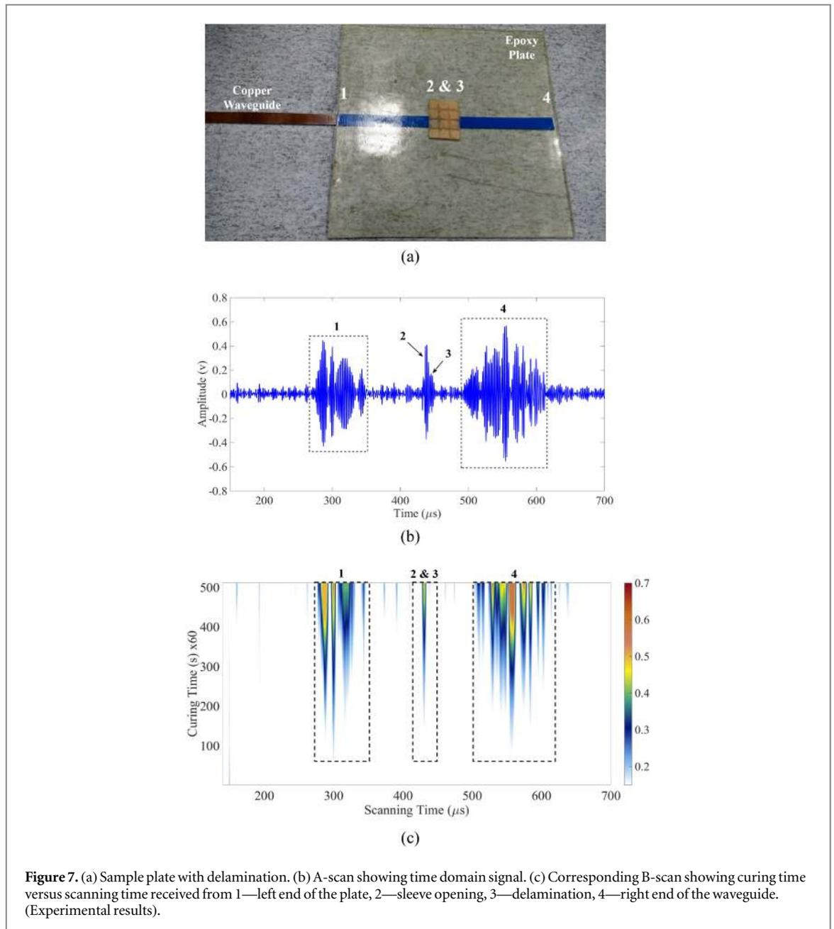
the change in impedance. In the case of delamination, leaked wave energy reflects back from delamination as well and travels back to the receiver and to the right end of the waveguide. Hence, in the case of delamination over sleeve opening, the reflection received from sleeve opening and the right end is higher than the case of no delamination. Figure 8 shows the energy variations for both the cases (with and without delamination) at the sleeve opening and at the right end of the waveguide.
