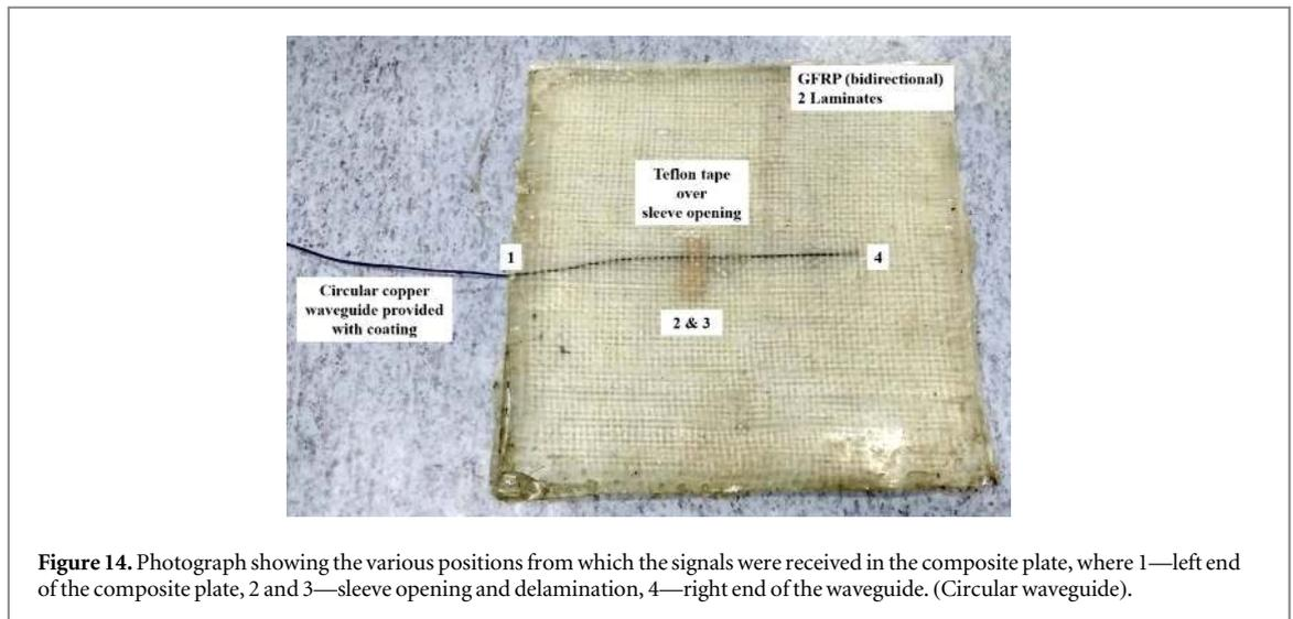
**Figure 14.** Photograph showing the various positions from which the signals were received in the composite plate, where 1—left end of the composite plate, 2 and 3—sleeve opening and delamination, 4—right end of the waveguide. (Circular waveguide).
