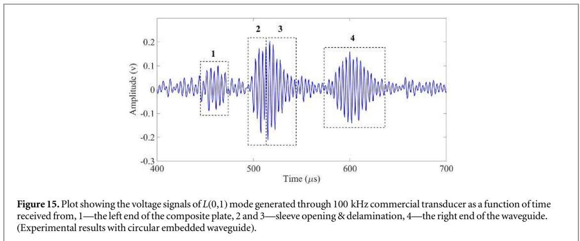
**Figure 15.** Plot showing the voltage signals of  $L(0,1)$  mode generated through 100 kHz commercial transducer as a function of time received from, 1—the left end of the composite plate, 2 and 3—sleeve opening & delamination, 4—the right end of the waveguide. (Experimental results with circular embedded waveguide).
