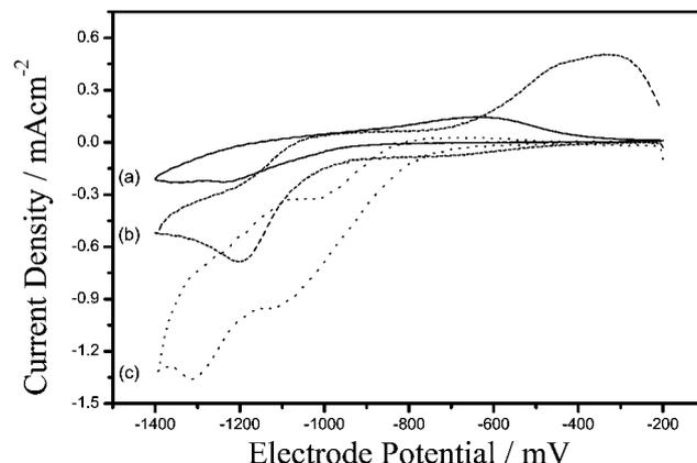
**Fig. 1** Cyclic voltammograms for the reduction of 2,4-DCP in 0.1 M  $\text{Na}_2\text{SO}_4$ - $\text{H}_2\text{SO}_4$  at a palladised titanium electrode for no DCP (a), 1 mM DCP (b) and 20 mM DCP (c). The scan rate was  $5$   $\text{mV s}^{-1}$  and the reference electrode was Ag/AgCl in  $\text{KCl}_{(\text{sat})}$  solution.
