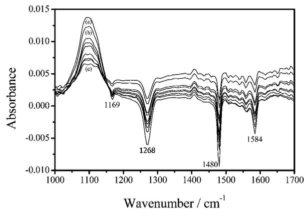
**Fig. 2** FTIR spectra for the dehalogenation of 2,5-DCP at palladised titanium electrode. The electrode was set to  $-1400$  mV and the spectra are presented with respect to the reference spectrum taken at 0 min; (a) 2 min; (b) 5 min, then every 5 min to 40 min (c).
