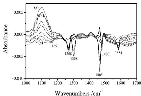
**Fig. 3** FTIR spectra for the dehalogenation of 2,4-DCP at palladised titanium electrode. The electrode was set to  $-1400$  mV and the spectra are presented with respect to the reference spectrum taken at 0 min; (a) 2 min; (b) 5 min, then every 5 min to 40 min (c).
