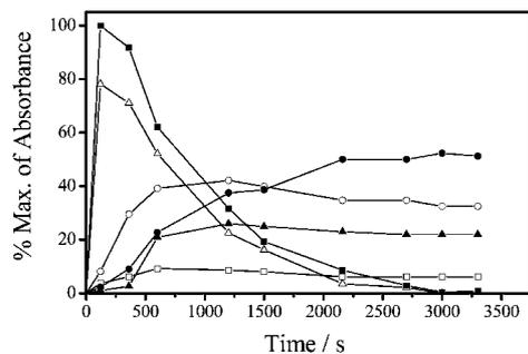
**Fig. 4** Plot of the peak intensities observed for 20 mM 2,4-dichlorophenol at  $-1400$  mV as a function of time for wave numbers 1169(□), 1268(○), 1308(△), 1465(■), 1480(●), 1584(▲)  $\text{cm}^{-1}$ .
