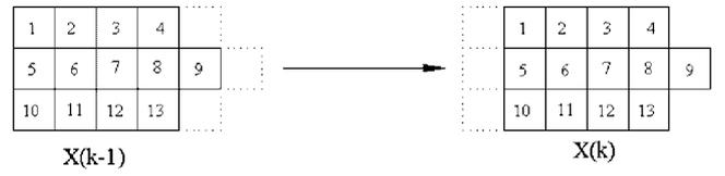
Fig. 2 State movement to the right by one block at every time step
