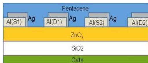
FIG. 1. (Color online) Schematic diagram of ambipolar hybrid organic/inorganic TFTs (dimensions are not scaled).
