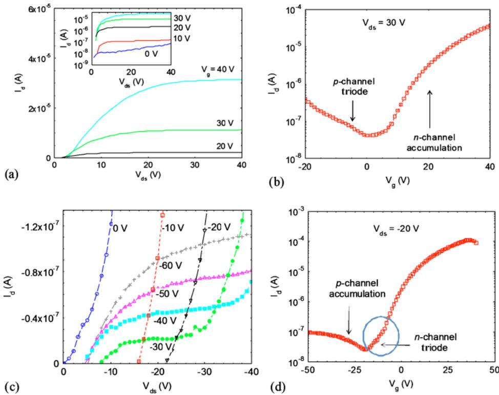
FIG. 2. (Color online) (a) Output and (b) transfer characteristics of hybrid TFTs under  $V_{ds} > 0$  ( $n$ -channel accumulation and  $p$ -channel triode modes). Inset of (a) shows output characteristics in semi logarithmic scale. (c) Output and (d) transfer characteristics of the device at  $V_{ds} < 0$  ( $p$ -channel accumulation mode and  $n$ -channel triode mode).
