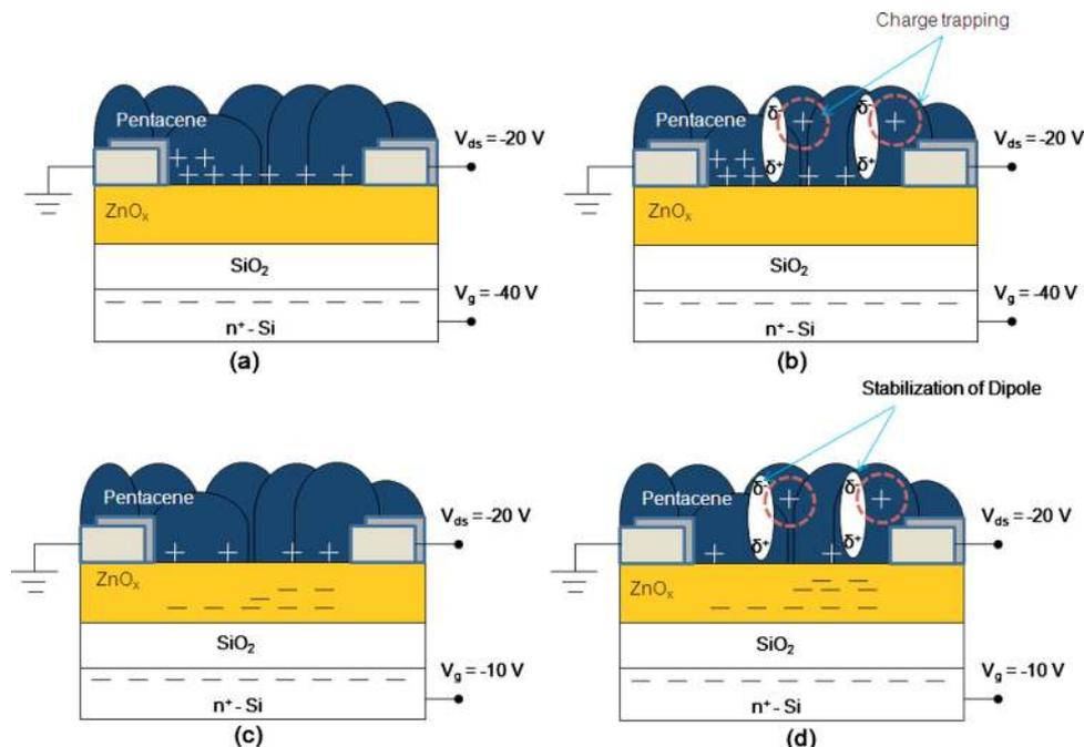
FIG. 4. (Color online) Schematic diagram of proposed mechanism in *p*-channel accumulation mode (a) before and (b) during analyte delivery and in *n*-channel triode mode (c) before and (d) during analyte delivery.
