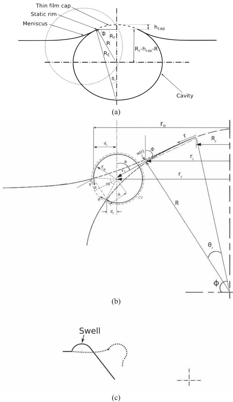
**FIG. 2.** (a) Schematic of the static bubble at the free surface; (b) zoomed-in view of the region within the dotted circle in (a), showing the retracted rim in the meniscus region with a bulge at its tip, creating an expanding hole at the free surface; and (c) movement of the swell.
