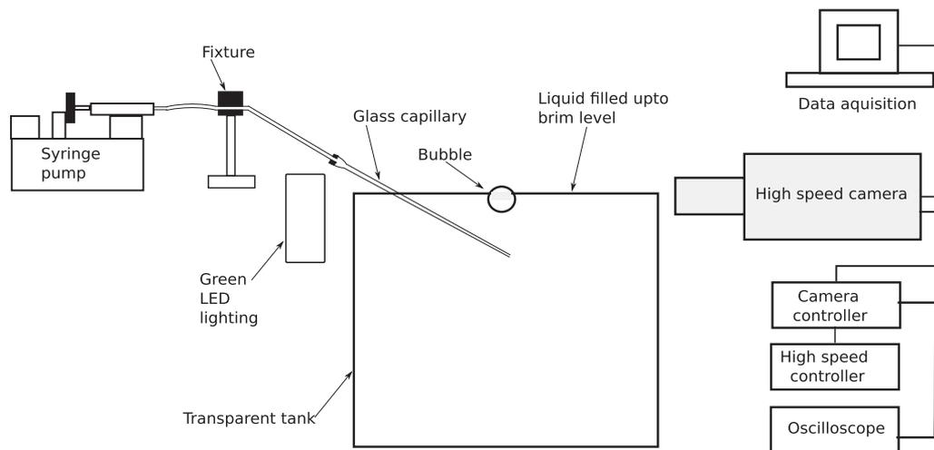
FIG. 3. Schematic of the experimental setup.
