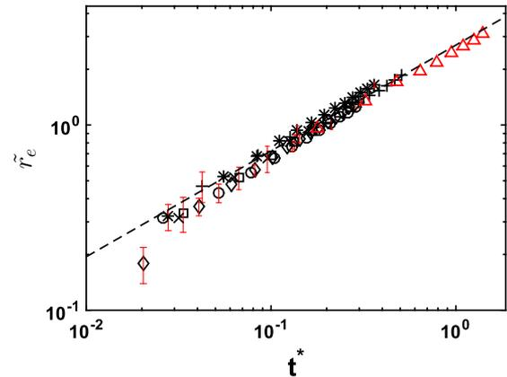
**FIG. 8.** Variation of the dimensionless excess outer radius of the rim  $\tilde{r}_e = r_e(t)/R$  with the dimensionless time  $t^* = t/t_c$ . For water: +,  $R = 0.175$  mm; \*,  $R = 0.47$  mm;  $\circ$ ,  $R = 2.32$  mm; and  $\square$ ,  $R = 1.47$  mm. For other fluids:  $\diamond$ ,  $R = 0.7$  mm, GW55;  $\times$ ,  $R = 1.16$  mm, ethanol;  $\triangle$ ,  $R = 25$   $\mu$ m, ethanol from San Lee *et al.*<sup>17</sup> and  $-$ ,  $\tilde{r}_e = 2.7 t^{*4/7}$  (31).
