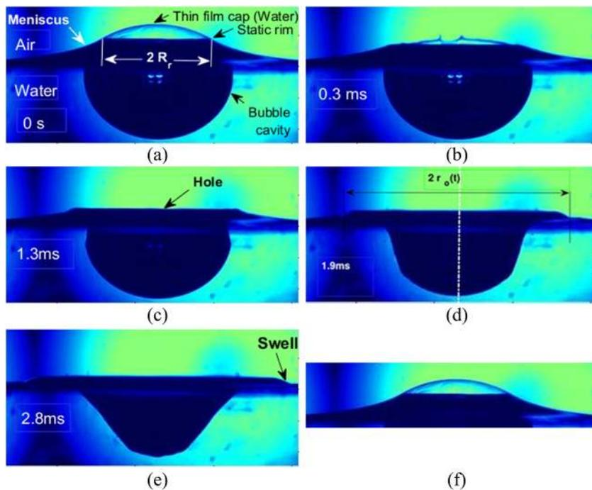
**FIG. 1.** Hole expansion at the free surface from a bubble of  $R = 2.32$  mm ( $Bo = 0.73$ ) in water. (a) The static bubble shape, (b) hole expansion in the thin film and its subsequent fragmentation, (c) hole expansion in the meniscus region, and [(d) and (e)] hole expansion along the free surface. Each image width is 9.2 mm. A movie showing a magnified view of hole expansion for the sequence is attached (f). Multimedia view: <https://doi.org/10.1063/1.5139569.1>
