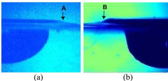
**FIG. 11.** Comparison of the swell in a high viscosity fluid with that in water at approximately 1.4 ms after the thin film rupture. (a) A smooth swell for  $R = 2.4$  mm ( $Oh = 0.27$ ,  $R/R_{\mu\sigma} = 13.7$ ) in GW86.8. Image width is 5.1 mm. (b) A sharp swell for  $R = 2.32$  mm ( $Oh = 0.0025$ ,  $R/R_{\mu\sigma} = 16 \times 10^4$ ) in water. Image width is 4.63 mm.
