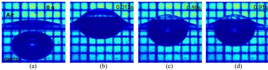
**FIG. 4.** The interaction of a rising bubble of  $R = 2.2$  mm ( $Bo = 0.9$ ) with the free surface in GW72. (a) Approach to the free surface, [(b) and (c)] oscillation at the free surface, and (d) the static configuration. For similar  $Bo$ , the bubble collapses 4 s after (d). Grid size is 1 mm.
