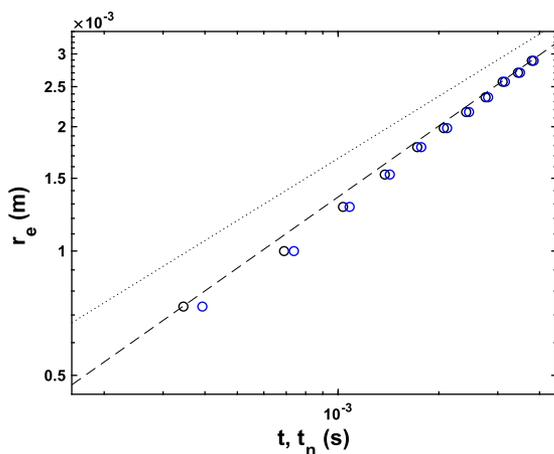
**FIG. 12.** Effect of uncertainty in the origin of time on the variation of the excess radius ( $r_e$ ) for  $R = 2.32$  mm in water. Black circles,  $r_e$  vs  $t$ , same as the data shown in Fig. 7; blue circles,  $r_e$  vs  $t_n$ , where  $t_n = t - \delta t$ ; --,  $0.07 t^{4/7}$ ; and . . . ,  $0.053 t^{1/2}$ .
