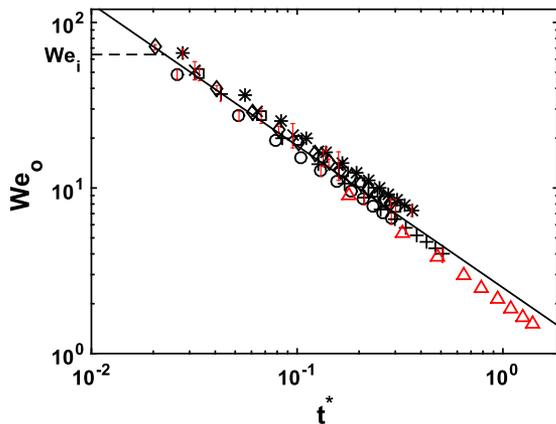
**FIG. 9.** Variation of the Weber number of expansion of the outer radius of the hole  $We_o$  with the dimensionless time  $t^* = tt_c$ . For water: +,  $R = 0.175$  mm; \*,  $R = 0.47$  mm; ○,  $R = 2.32$  mm; and □,  $R = 1.47$  mm. For other fluids: ◇,  $R = 0.7$  mm, GW55; ×,  $R = 1.16$  mm, ethanol; △,  $R = 25$  μm, ethanol from San Lee *et al.*;<sup>17</sup> —,  $We_o = 2.5t^{*-6/7}$  (34); and - - ,  $We_i = 64$  (38).
