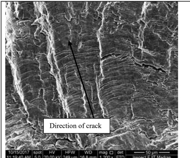
**Fig. 12.** Observed striation pattern for SS316 MP-TIG joint, located 12mm from initiation zone.
