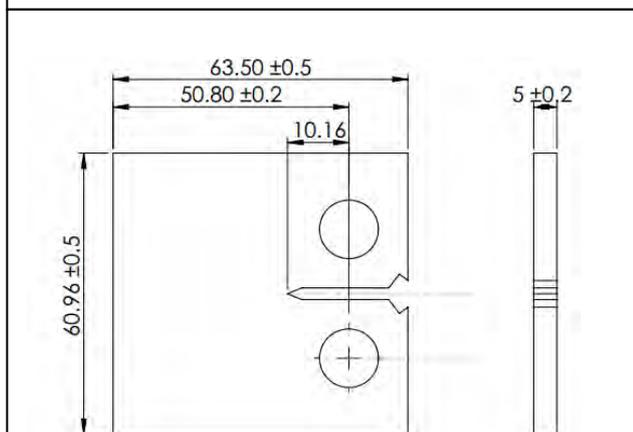
**Fig. 2.** Schematic of C(T) specimen. All dimensions are in mm.
