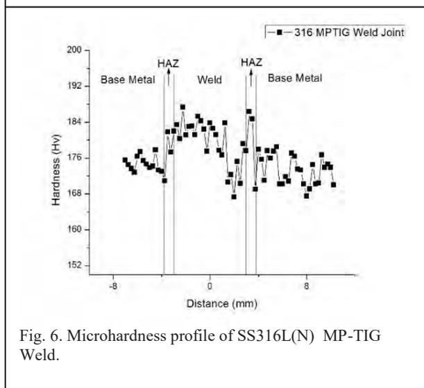
Fig. 6. Microhardness profile of SS316L(N) MP-TIG Weld.
