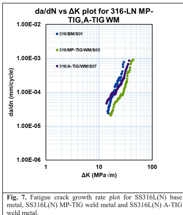
Fig. 7. Fatigue crack growth rate plot for SS316L(N) base metal, SS316L(N) MP-TIG weld metal and SS316L(N) A-TIG weld metal.
