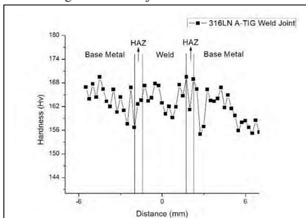
Fig. 5. Microhardness profile of SS316L(N) A-TIG Weld.
