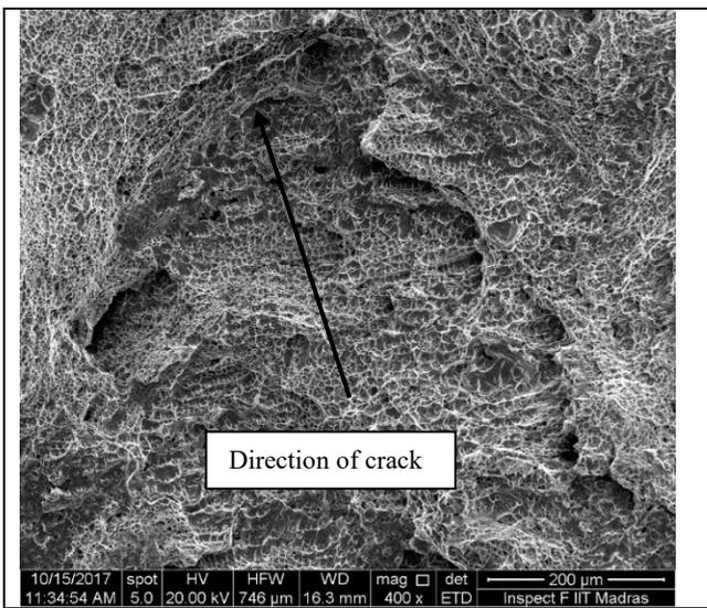
**Fig. 13.** Final fracture surface observed for SS316L(N) MP-TIG
