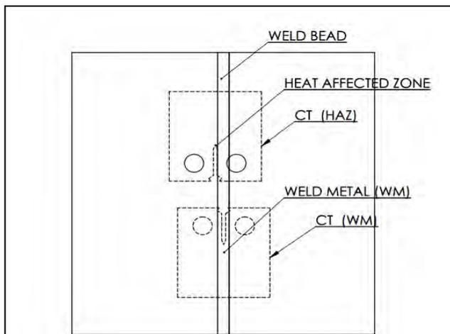
**Fig. 1.** Compact tension specimen extraction lay out from weld plates.
