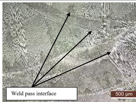
**Fig. 4.** Microstructure of SS316L(N) MP-TIG Weld.
