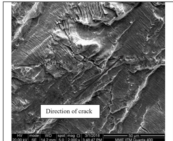
**Fig. 11.** Observed striation pattern for SS316L(N) A-TIG joint, located at ~10mm from initiation zone.
