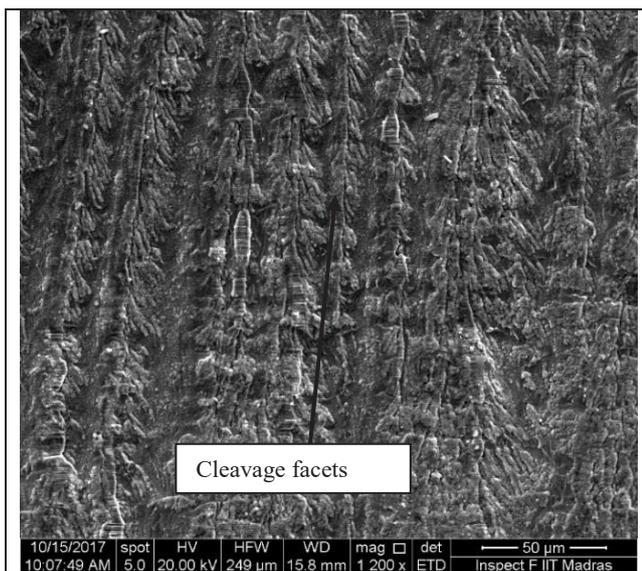
**Fig. 9.** Trans-granular cleavage facets observed in SS316L(N) MP-TIG welds, at a distance of ~2 mm from initiation ( $\Delta K \sim 15 \text{ MPa}\sqrt{\text{m}}$ )
