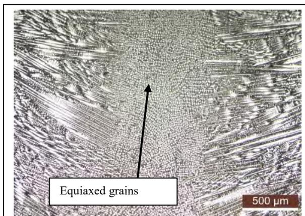
**Fig. 3.** Weld Microstructure of SS316L(N) A—TIG Weld.
