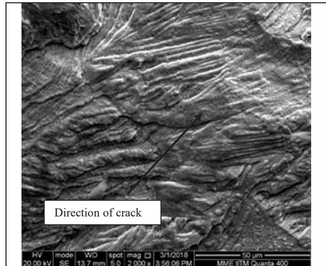
**Fig. 10.** River line pattern of fracture surface for SS316 A-TIG joint, located at a distance of ~2 mm from the Chevron notch initiation zone.
