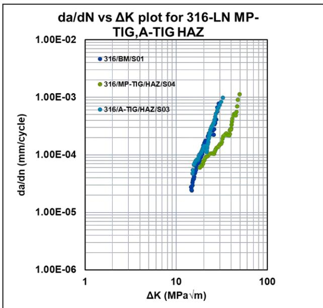
**Fig. 8.** Fatigue crack growth rate plot for SS316L(N), SS316L(N) MP-TIG weld and SS316L(N) A-TIG in the Heat Affected Zone.
