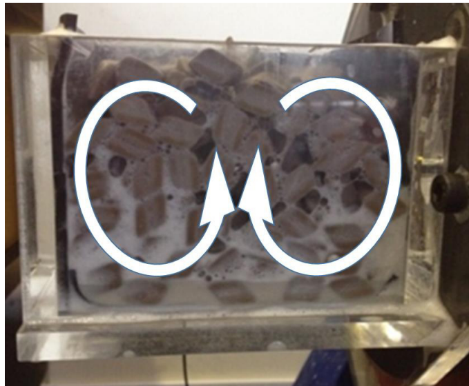
Figure 7. Media motion in clockwise direction and anti-clock wise direction as seen through acrylic bowl
