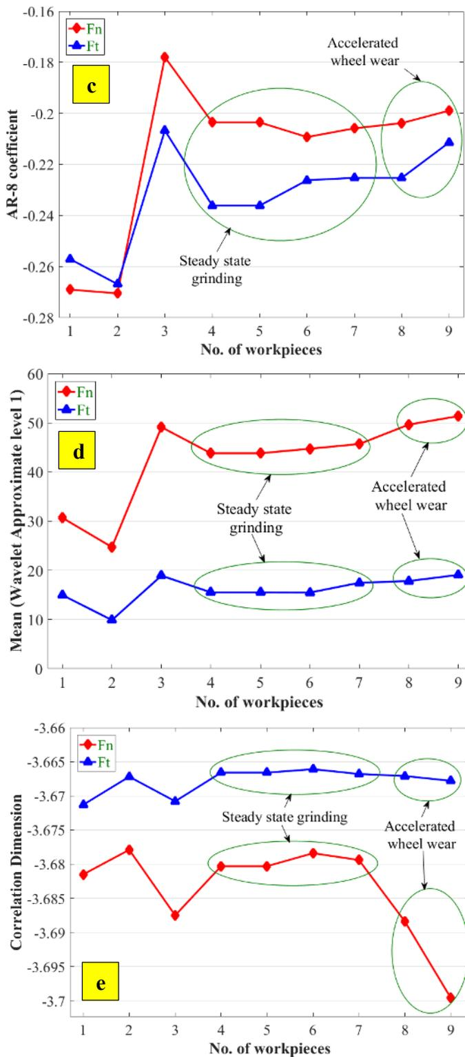
Fig. 5. Effective grinding force features: (a) Energy; (b) Mean; (c) AR-8 coefficient; (d) Mean wavelet level 1 approximate coefficient; (e) Correlation dimension
