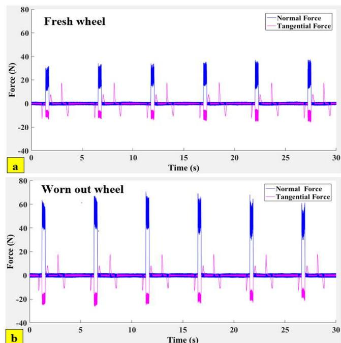
Fig. 4. Grinding Forces: (a) Fresh wheel; (b) Worn-out wheel
