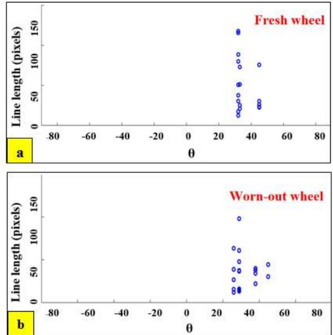
Fig. 8. Detection of line length and orientation: (a) Fresh wheel; (b) Worn-out wheel
