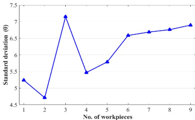
Fig. 10. Standard deviation of line orientation variation over number of ground workpiece
