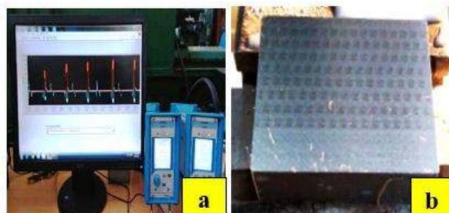
Fig. 3. (a) Grinding force signal acquisition; (b) Workpiece surface burn mark
