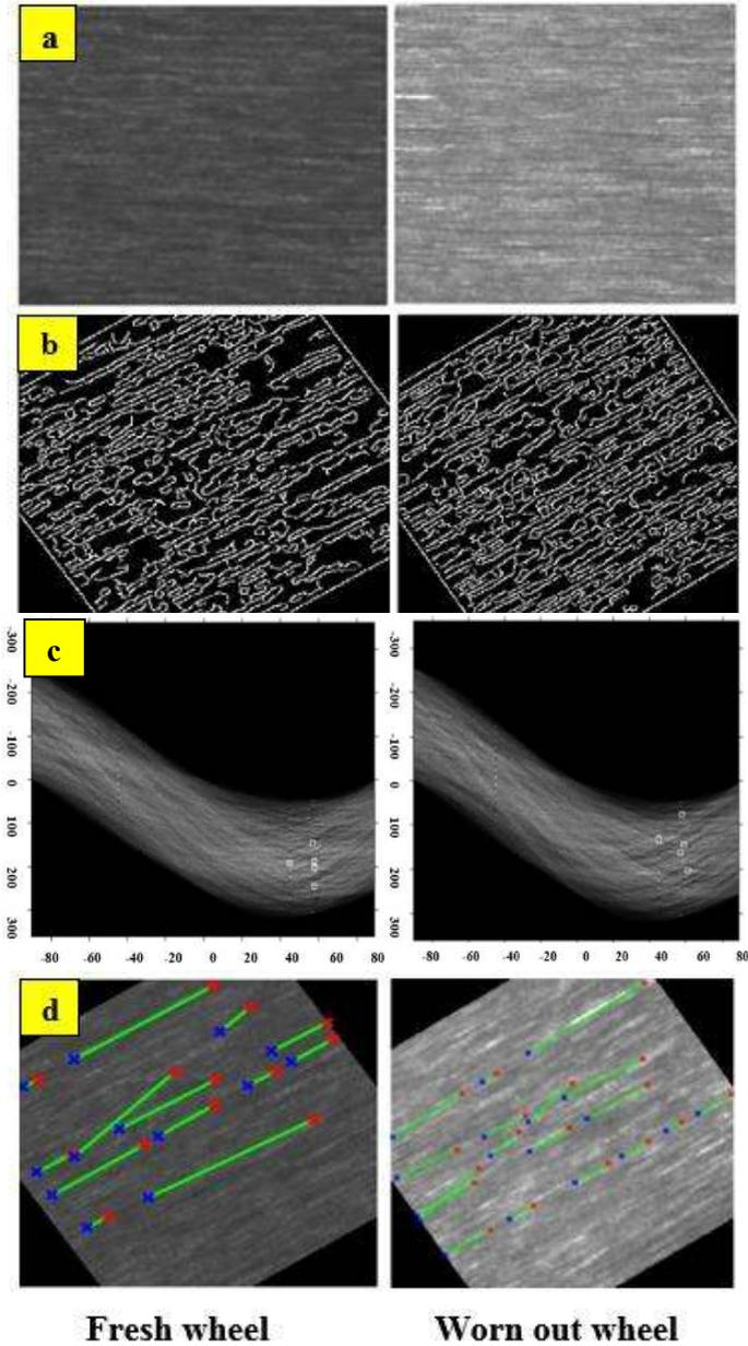
Fig. 7. Fresh and worn out wheel: a) Cropped ground surface image; b) Canny edge image; c) Hough transform (parameter space); d) Detected line segments
