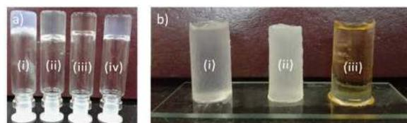
**Fig. 3** a) Inverted vials showing immobilized gels of **1.4** from (i) n-Heptane (2 wt%), (ii) Diesel (2 wt%), (iii) Tetralin (2.5 wt%), (iv) CCl<sub>4</sub> (2.5 wt%); b) its self-standing gels from i) Mesitylene, ii) CCl<sub>4</sub>, iii) Tetralin.
