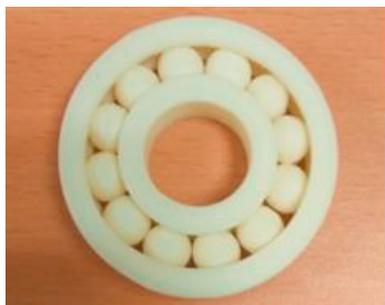
Fig. 12 Bearing printed using ABS
