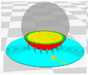
Fig. 4 Line Support Structure
