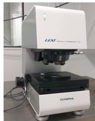
Fig. 7 Confocal microscope used for measuring the Sa values
