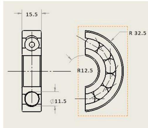
Fig. 2 2D drawing of the assembly (Dimensions in mm)
