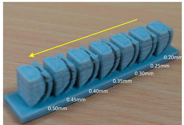
Fig. 3 Calibration model for clearance feature. Arrow shows the direction in which clearance increases
