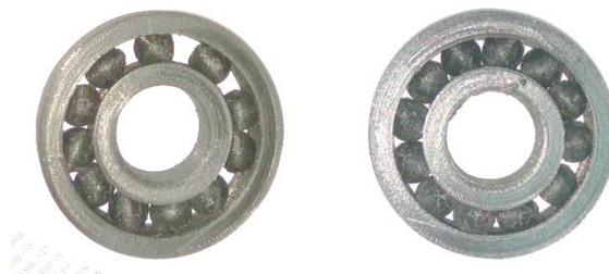
Fig. 9 Bearing printed using PLA with: 11 Balls(Left) and 12 Balls (Right)
