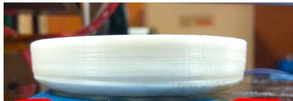
Fig. 10 Nylon 66 sample warped in the base
