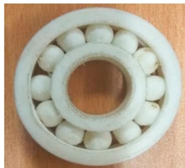
Fig. 11 Bearing printed using Nylon 6 6
