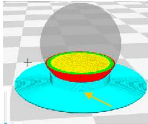
Fig. 5 Grid Support Structure
