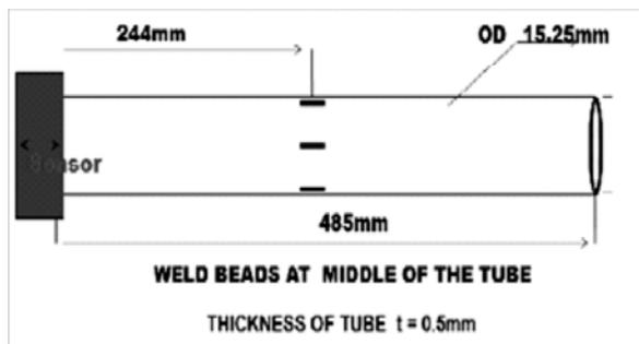
Fig. 4 : Dimensions of the fuel tube
