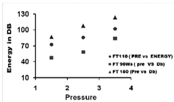
Fig. 9 : Shows the Energy of the reflected signal vs. Applied Pressure and Power to the electrodes for the 9 welded tubes of sample set 2.
