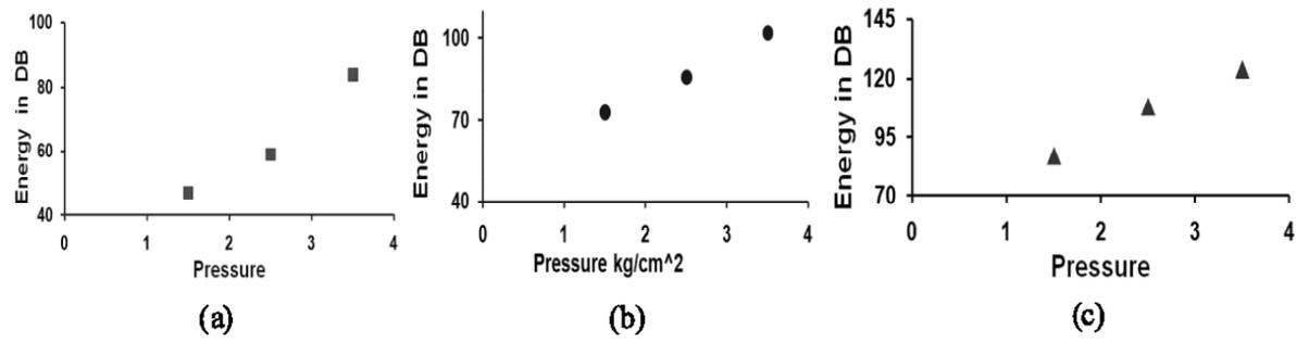
Fig. 8 : Pressure vs. reflected energy from welded tube based on table 2. (a). 90Ws, (b).110Ws, (c).150Ws
