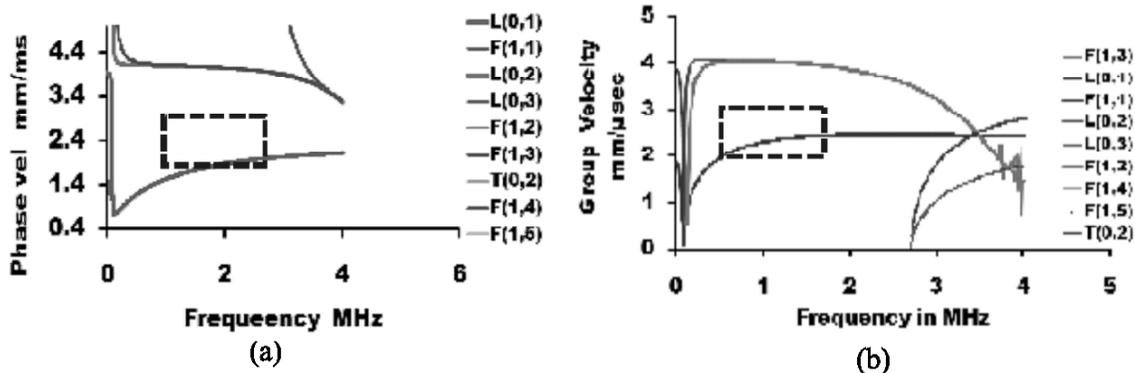
Fig. 2 : Dispersion curves for Zircalloy-4 tube (diameter 15.25mm and thickness 0.5 mm) (a) phase velocity, and (b) group velocity plots.
