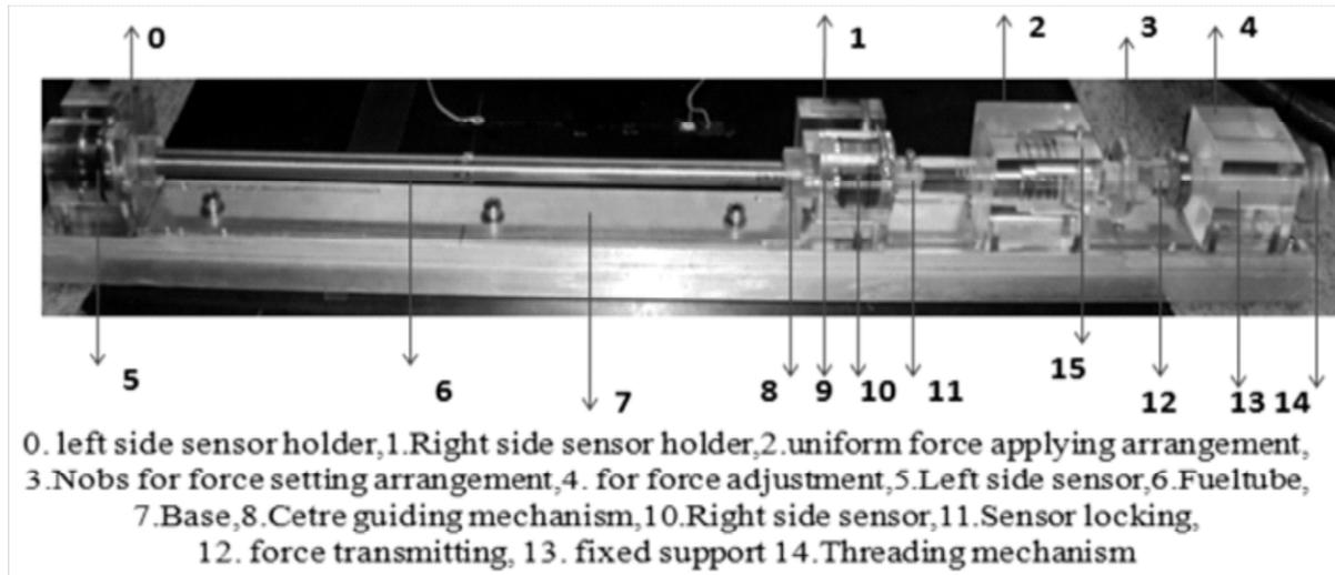
Fig. 3 : Photograph of the experimental setup used for generation and reception of guided waves.
