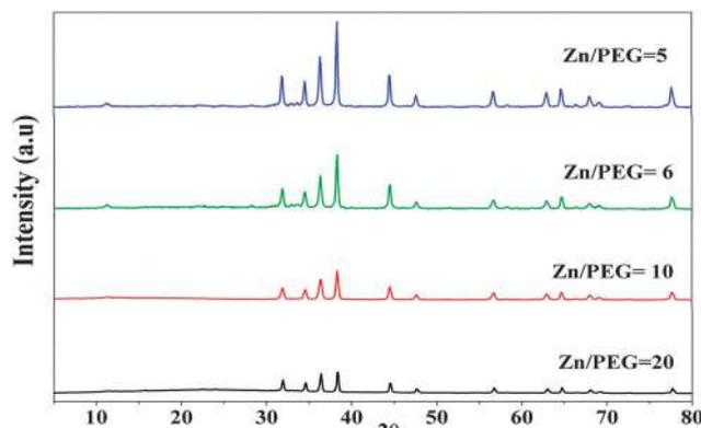
Fig. 2 X-ray diffraction patterns of calcined 5% Au-ZnO nanocomposites prepared at different Zn/PEG ratios.
