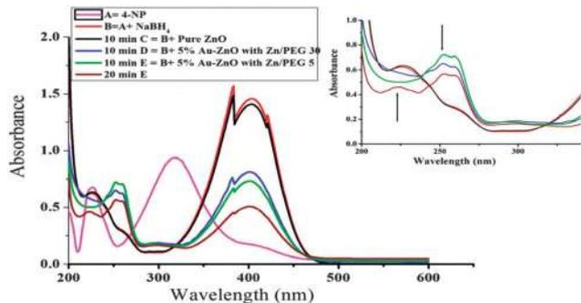
Fig. 13 UV-visible spectra of the reduction of 4-NP with  $\text{NaBH}_4$  in the presence of Au-ZnO nanocomposites at different time intervals. Inset: enlarged UV-visible spectra showing time dependent formation of intermediate ( $\downarrow$ ) 4-aminophenolate anion and 4-aminophenol ( $\uparrow$ ).
