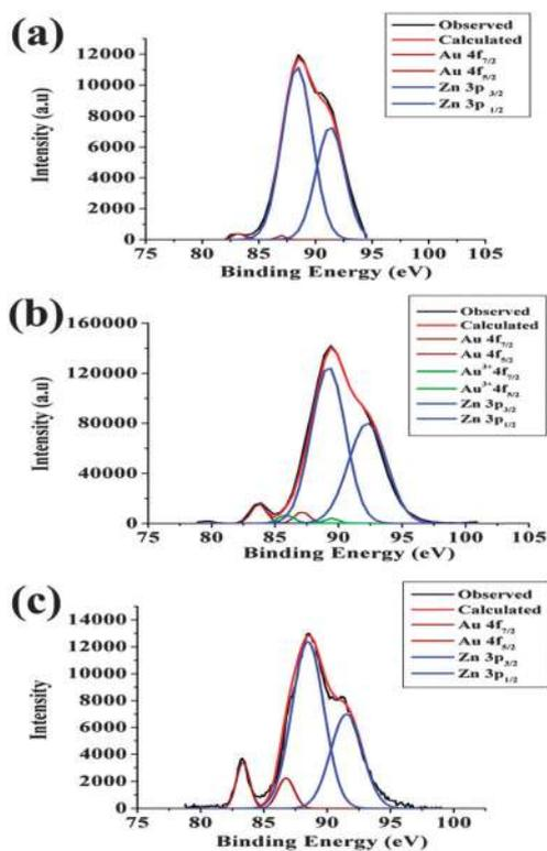
Fig. 3 Photoelectron spectra of Au–ZnO: (a) 0.5% Au–ZnO prepared at a Zn/PEG ratio of 30; (b) 5% Au–ZnO prepared at a Zn/PEG ratio of 30 and (c) 5% Au–ZnO prepared at a Zn/PEG ratio of 5.
