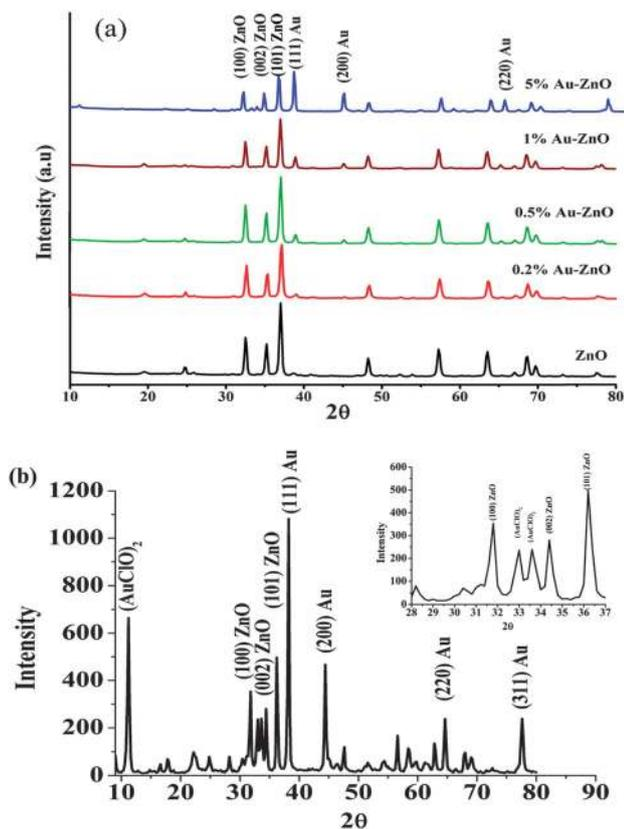
Fig. 1 (a) X-ray diffraction patterns of pure ZnO and Au-ZnO nanocomposites prepared at a Zn/PEG ratio of 30, (b) X-ray diffraction pattern of pre-calcined 5% Au-ZnO. The inset picture shows the enlarged XRD peaks between  $2\theta = 30$  and  $36$ .
