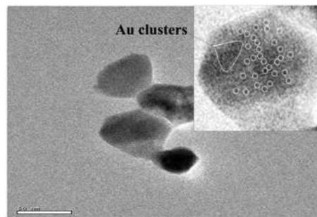
Fig. 7 TEM image of 5% Au–ZnO prepared at a Zn/PEG ratio of 5. The inset picture with rounded dark spots gives the enlarged image showing the presence of Au clusters.
