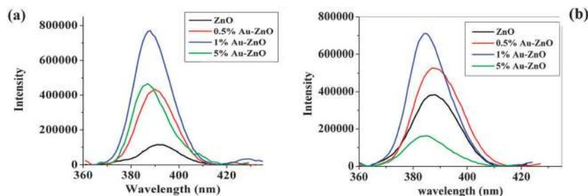
Fig. 12 Photoluminescence spectra of pure and Au–ZnO nanocomposites prepared at Zn/PEG ratios of (a) 30 and (b) 5.
