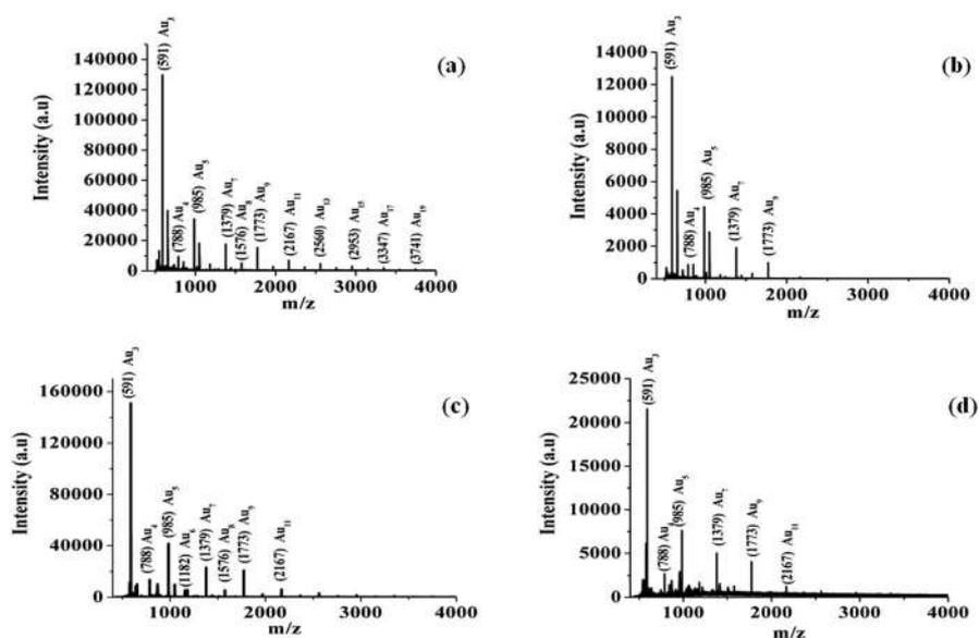
Fig. 10 MALDI-TOF mass spectra (positive ions) of 5% Au–ZnO prepared at Zn/PEG ratios of (a) 10, (b) 6 and (c) 5 and (d) MALDI-TOF mass spectra (positive ions) of 1% Au–ZnO prepared at a Zn/PEG ratio of 5.
