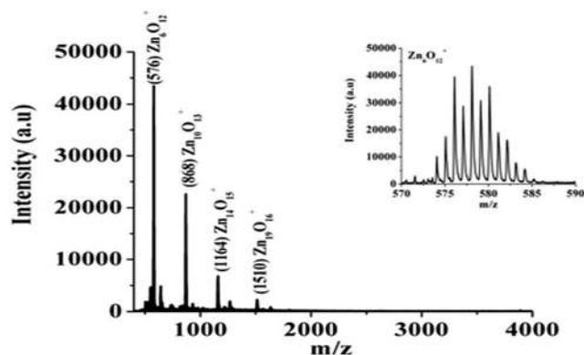
Fig. 8 MALDI-TOF mass spectra (positive ions) of pure ZnO. Inset: isotropic distribution of  $\text{Zn}_6\text{O}_{12}^+$ .
