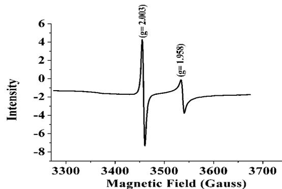
Fig. 4 Room temperature electron paramagnetic resonance of 5% Au–ZnO nanocomposites prepared at a Zn/PEG ratio of 6.
