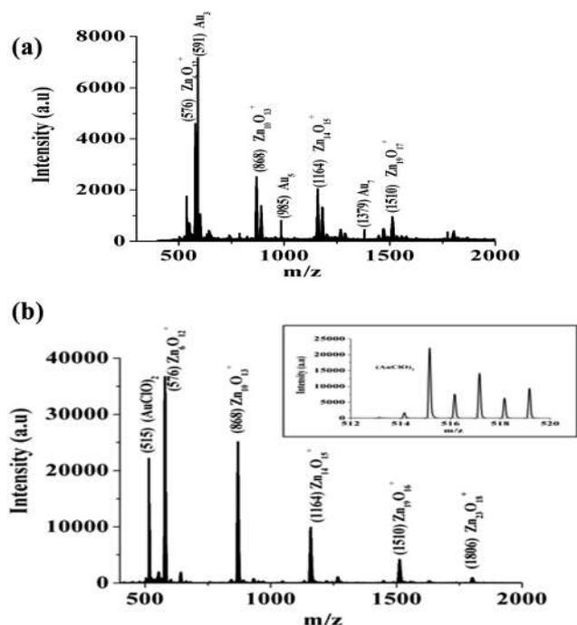
Fig. 9 MALDI-TOF mass spectra (positive ions) of Au–ZnO prepared at a Zn/PEG ratio of 30 at different Au concentrations: (a) 1% Au and (b) 5% Au. Inset in (b): isotropic distribution of  $(\text{AuClO})_2$  due to  $^{35,37}\text{Cl}$ .
