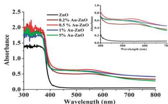
Fig. 11 DRS UV-Vis spectra of pure and Au-ZnO nanocomposites at a Zn/PEG ratio of 30. The inset showing a compressed spectrum is intended to bring out the clarity of the SP band.
