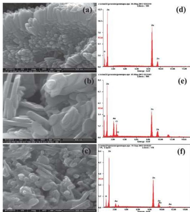
Fig. 5 SEM images of (a) ZnO (calcined) and (b) 5% Au–ZnO both with a Zn/PEG ratio of 30 (precalcined) and (c) calcined 5% Au–ZnO with a Zn/PEG ratio of 5, and their corresponding EDX (d–f).
