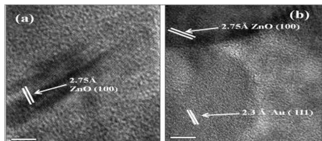
Fig. 6 HRTEM image of (a) pure ZnO with Zn/PEG of 30 and (b) 5% Au–ZnO with Zn/PEG of 5.
