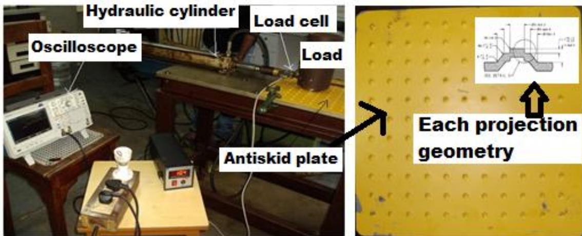
**Figure 1.** Experimental setup for friction test
