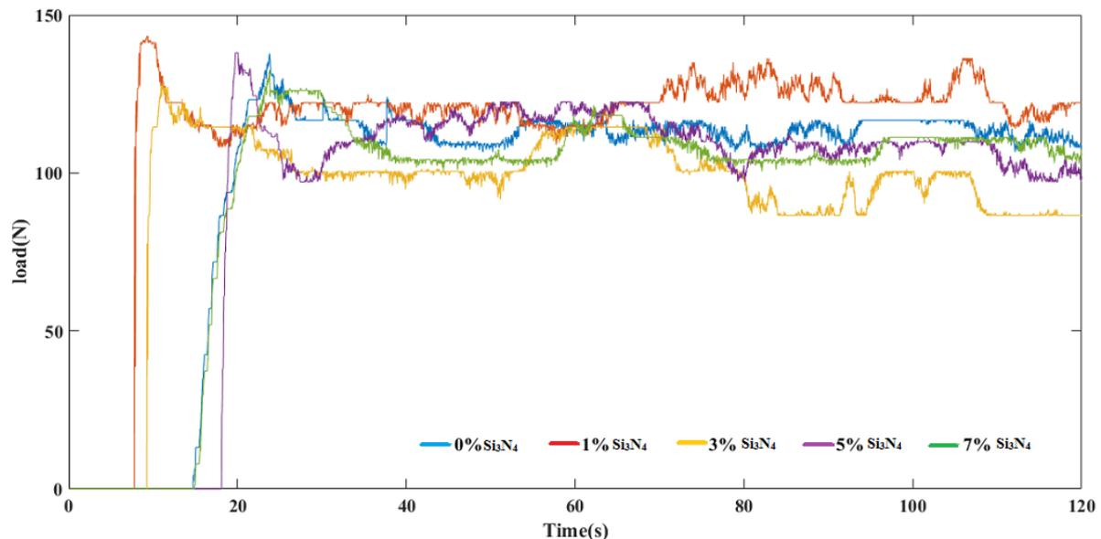
**Figure 7. Load - time plot for friction test at dry condition**
