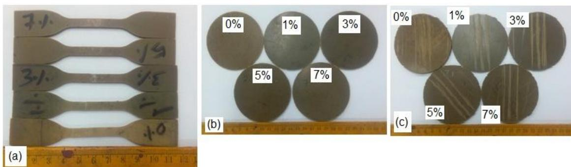
**Figure 2.** (a) Tensile test Specimens (b) Specimens-before friction testing (c) Friction tested specimens
