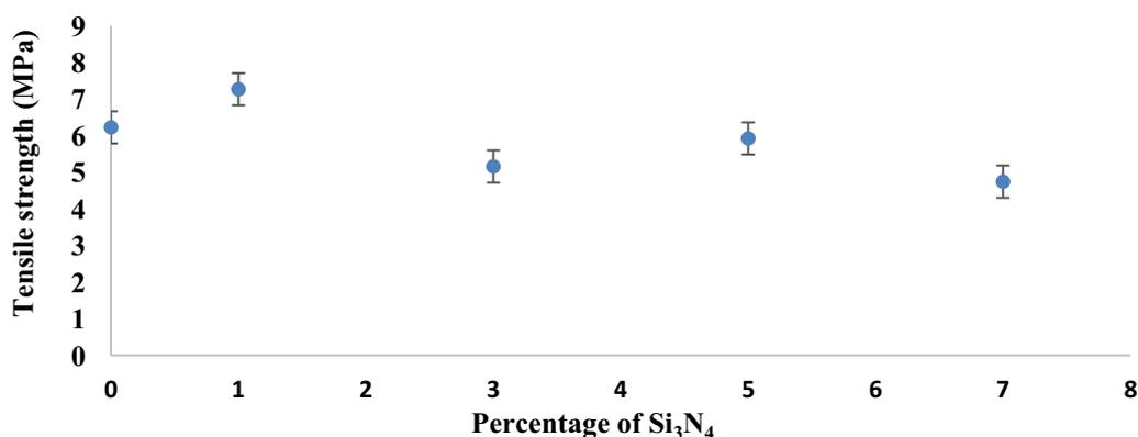
**Figure 4.** Tensile strength of NR/SBR compounds with and without Si<sub>3</sub>N<sub>4</sub>
