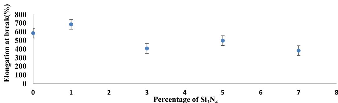
**Figure 6.** Elongation percentage of NR/SBR compounds with and without Si<sub>3</sub>N<sub>4</sub> at the time of failure
