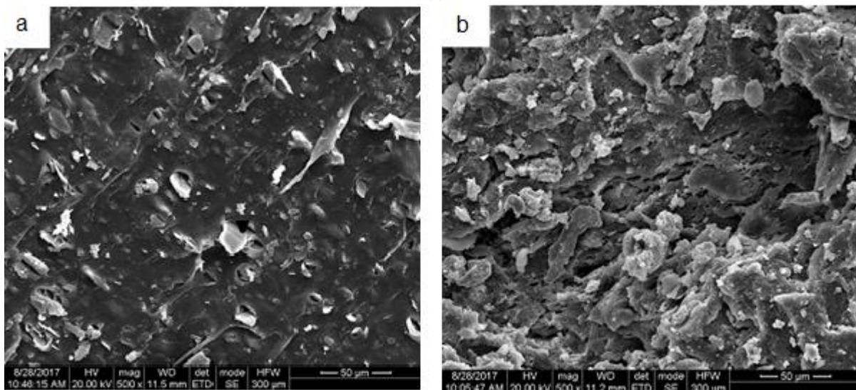
**Figure 9.** SEM micrograph of rubber specimen with 1% filler (a) before friction test (b) after friction test
