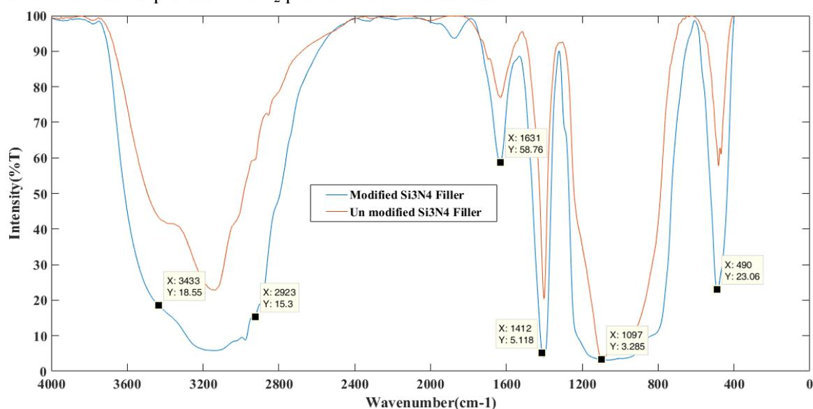
**Figure 3.** FTIR spectra of modified  $\text{Si}_3\text{N}_4$  and unmodified  $\text{Si}_3\text{N}_4$
