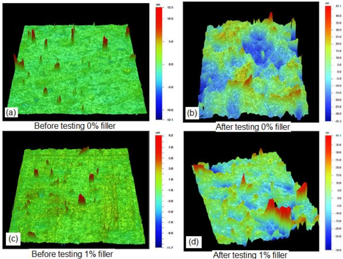
**Figure 10.** Surface topography of NR/SBR composites before friction test (a) without filler before testing (b) without filler after testing (c) with 1% filler before testing (d) with 1% filler after testing
