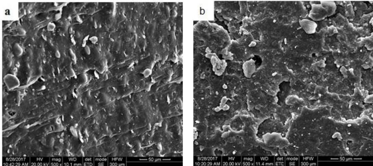
**Figure 8.** SEM micrograph of rubber specimen without filler (a) before friction test (b) after friction test
