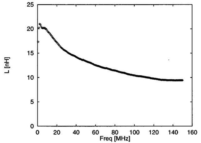
FIG. 2. Frequency dependence of the yoke inductance at zero dc write current. Yoke inductance is measured as the difference between the unsaturated and saturated write head inductance. The asymptotic value of  $L$  represents the inductance of the air coil with the yoke completely saturated.
