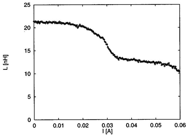
FIG. 1. Write current dependence of the yoke inductance. Yoke inductance is measured as the difference between the unsaturated and saturated write head inductance. The frequency of the small amplitude ac signal was 2 MHz.
