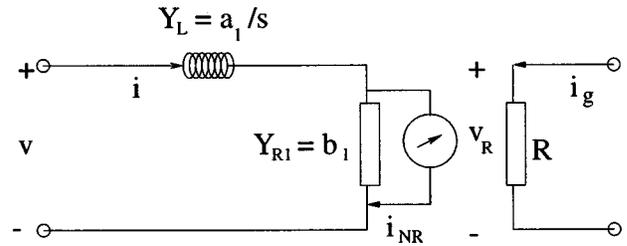
FIG. 5. Nonlinear lumped element circuit for a thin film write head. The input  $v(t) \equiv \text{MMF}$ , the current  $i(t) \equiv \phi$ , and the deep gap flux  $i_g(t) \propto v_R(t)$ .
