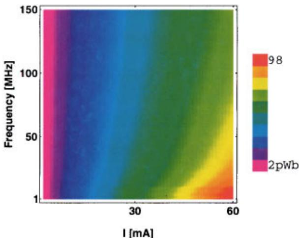
FIG. 4. Variation in yoke flux, as defined by Eq. (4), with changing input dc write current amplitude and ac write current frequency. The data were collected by sweeping frequency in steps of 0.75 MHz and then stepping up dc write current in steps of 1 mA.
