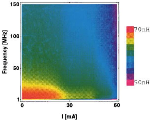
FIG. 3. Variation in unsaturated yoke inductance as a function of input dc write current amplitude and ac write current frequency.
