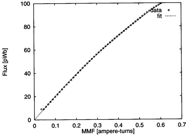
FIG. 6. Change in flux enclosed by the write coils as a function of input MMF, calculated by applying Eq. (4) to the data in Fig. 1. The dashed line is a least squares quadratic fit through the data points, corresponding to Eq. (8).
