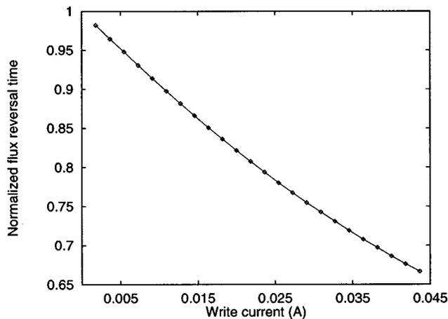
FIG. 7. Amplitude dependence of flux reversal time (10%–90% of maximum flux). The calculation is for reduced time,  $t' = t/\tau$ , and assumes a step input write current.
