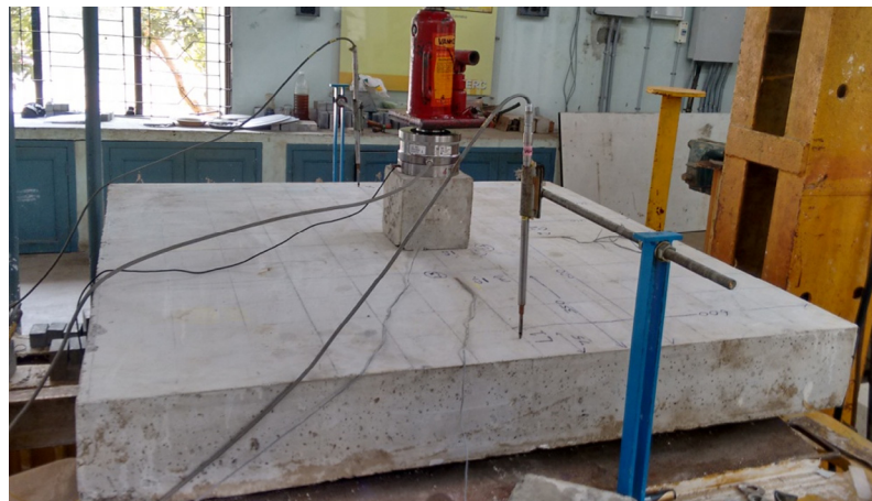
Figure 6 Photograph of panel ready for testing under punching load.
