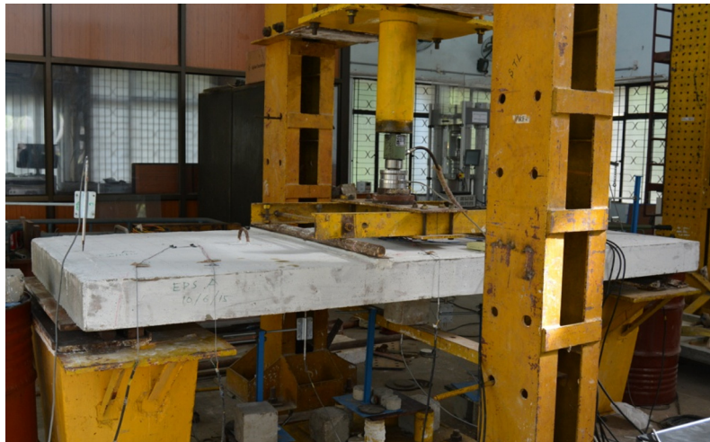
Figure 7 Photograph of panel ready for testing under four-point bending.
