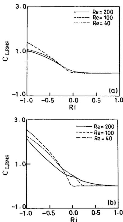
**Figure 11.** Variation of root mean square (RMS) lift coefficient against Richardson number (Ri) (a) upstream cylinder (b) downstream cylinder
