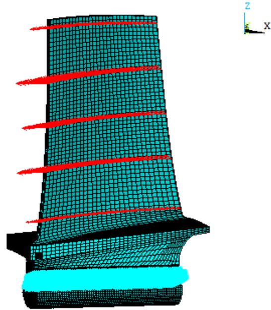
**Figure 3.** Loads and boundary conditions of compressor rotor blade
