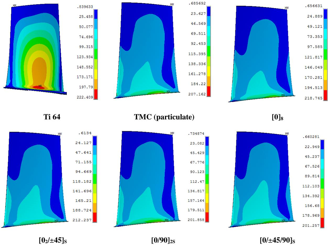
**Figure 5.** von Mises stress plot (MPa) of compressor rotor blade
