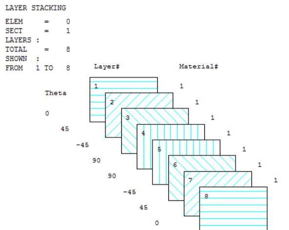
**Figure 4.** Sequence of lay up of composite laminate
