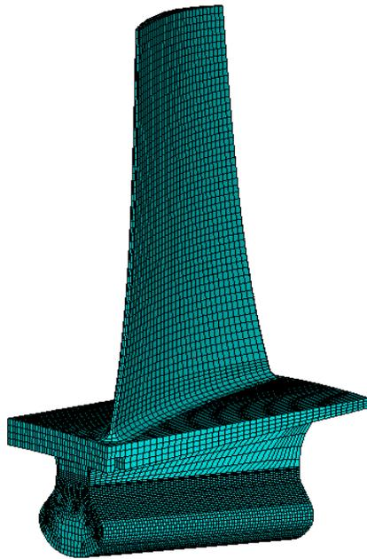
**Figure 2.** Finite element model of the compressor rotor blade
