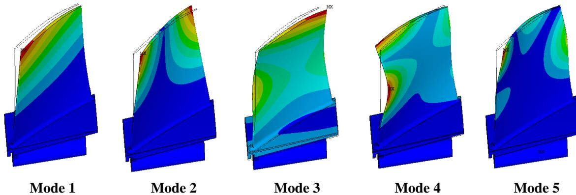
**Figure 6.** Mode shapes of Ti particulate composite rotor blade
