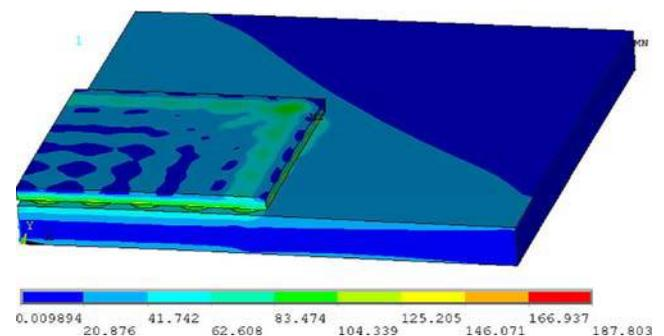
**Figure 18** Principal stresses in the flip-chip assembly (MPa)
