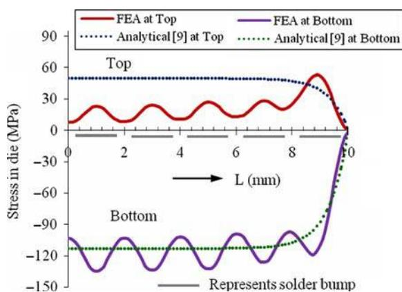
Figure 15 Bending stresses in substrate along top and bottom lines in  $x$ -axis direction
