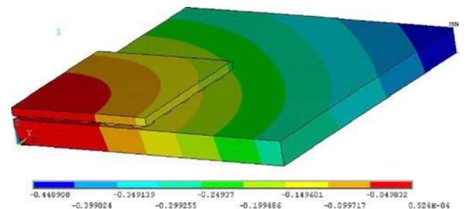
Figure 17 von Mises stresses in flip-chip assembly (MPa)
