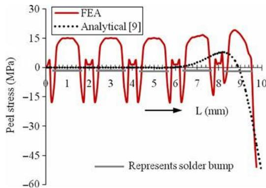
Figure 14 Bending stresses along top and bottom lines of the die in  $x$ -axis direction
