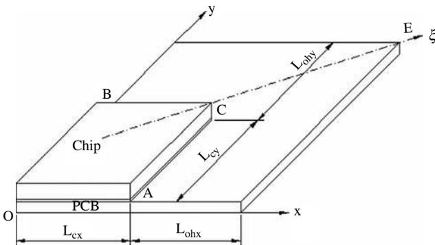
Transverse displacement of point C is equal to the sum of displacements of points A and B (Figure 6); for the square die these displacements are identical ( $x_C = x_A = y_C = y_B$  and  $w_A = w_B$ ) and therefore  $w_C = 2w_A$ , i.e.:
