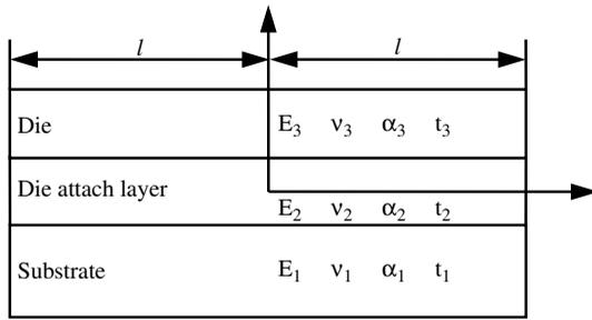
Figure 5 Free body diagram under thermal loading
