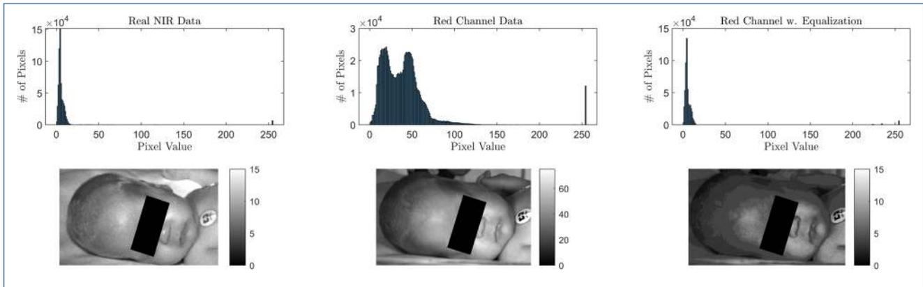
**Fig. 3** Left: Real NIR data. Center: Red channel of RGB image. Right: Virtual NIR image. The top row shows histograms; the bottom row excerpts of the corresponding images. Note the different scale of the colorbar in the center image
